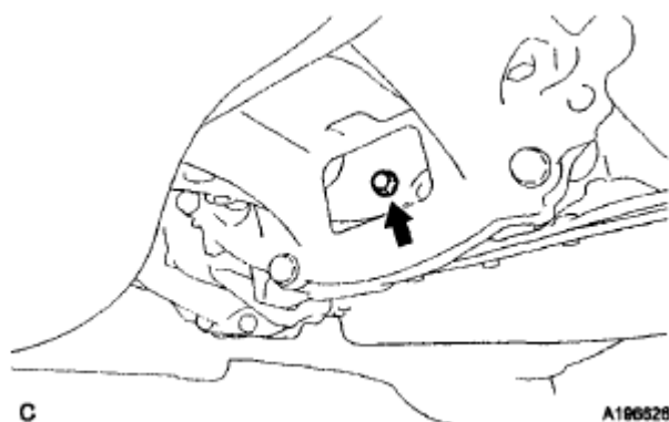
Fig. 271: Locating Torque Converter Clutch Setting Bolt Courtesy of TOYOTA MOTOR SALES, U.S.A., INC.
