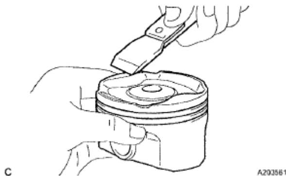
Fig. 140: Removing Carbon From Piston Top Courtesy of TOYOTA MOTOR SALES, U.S.A., INC.
