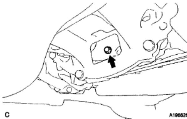
Fig. 246: Locating Torque Converter Clutch Setting Bolt
