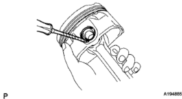
Fig. 133: Prying Out Snap Ring On Front Side
