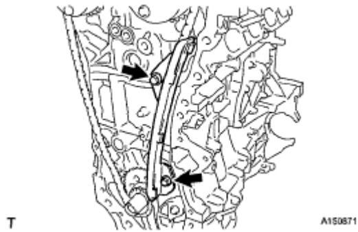
Fig. 89: Locating Bolts And No. 1 Chain Vibration Damper Courtesy of TOYOTA MOTOR SALES, U.S.A., INC.
