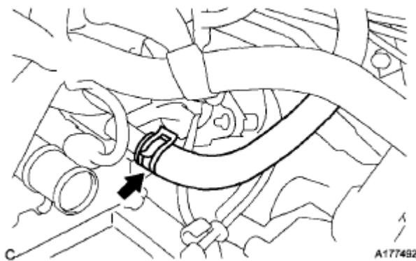
Fig. 148: Locating Inlet Heater Water Hose Clamp Courtesy of TOYOTA MOTOR SALES, U.S.A., INC.
