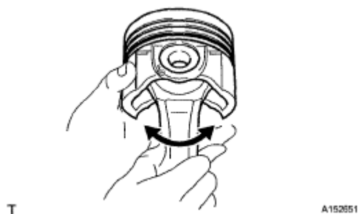
Fig. 455: Checking Fitting Condition Between Piston And Piston Pin Courtesy of TOYOTA MOTOR SALES, U.S.A., INC.
