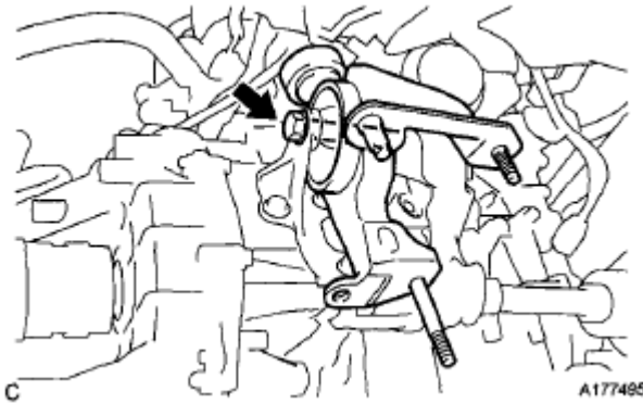
Fig. 170: Identifying Engine Mounting Bracket With Bolt Courtesy of TOYOTA MOTOR SALES, U.S.A., INC.
