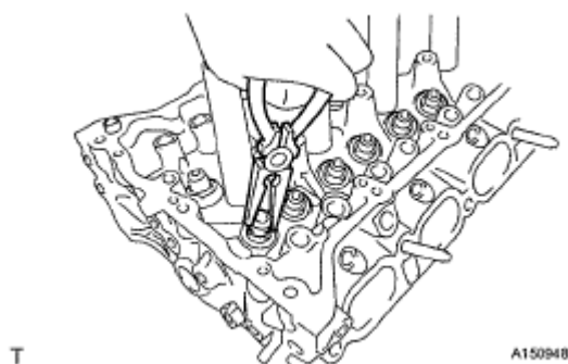
Fig. 363: Removing Valve Stem Oil Seal Courtesy of TOYOTA MOTOR SALES, U.S.A., INC.
