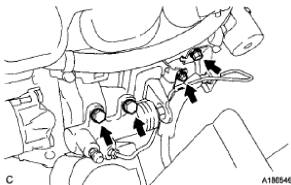
Fig. 153: Locating Clutch Tube Bracket Bolts Courtesy of TOYOTA MOTOR SALES, U.S.A., INC.
