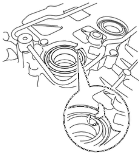
Fig. 294: Identifying Claws Of Baffle Plate
