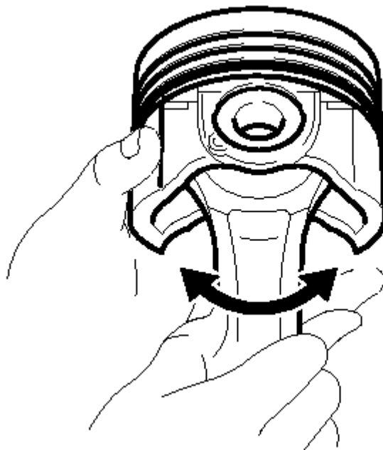
Fig. 464: Checking Fitting Condition Between Piston And Piston Pin Courtesy of TOYOTA MOTOR SALES, U.S.A., INC.
