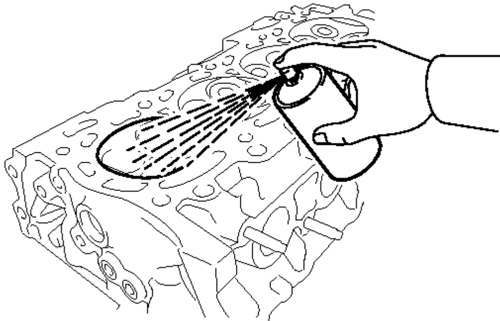
Fig. 374: Inspecting Cylinder Head For Cracks
