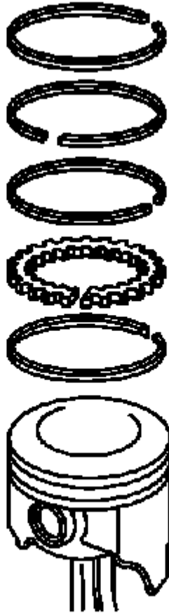
Fig. 519: Exploded View Of Piston Rings Courtesy of GENERAL MOTORS CORP.
