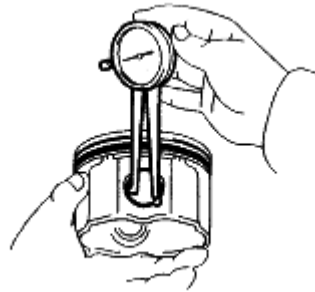
Fig. 372: Identifying Piston Pin Oil Clearance
