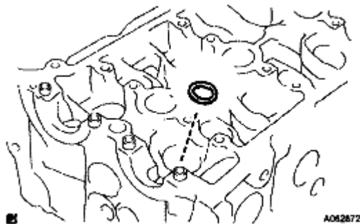
Fig. 162: Identifying Valve Spring Seat Courtesy of TOYOTA MOTOR SALES, U.S.A., INC.
