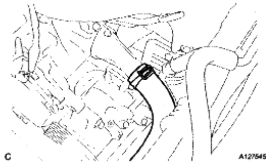
Fig. 213: Identifying Radiator Hose Outlet And Clamps Courtesy of TOYOTA MOTOR SALES, U.S.A., INC.
