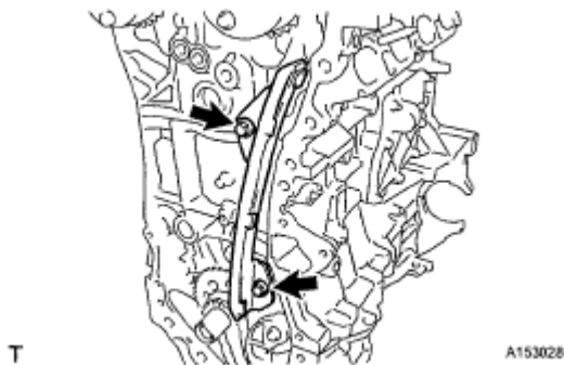
Fig. 94: Locating No. 1 Chain Vibration Damper Bolts Courtesy of TOYOTA MOTOR SALES, U.S.A., INC.
