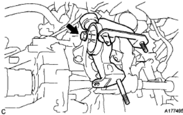
Fig. 159: Locating Rear Engine Mounting Insulator Courtesy of TOYOTA MOTOR SALES, U.S.A., INC.
