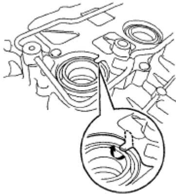
Fig. 283: Identifying Spark Plug Tube Gasket Courtesy of TOYOTA MOTOR SALES, U.S.A., INC.
