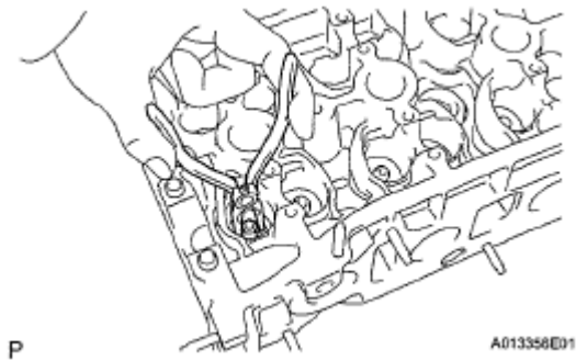
Fig. 342: Removing Valve Stem Oil Seal Courtesy of TOYOTA MOTOR SALES, U.S.A., INC.
