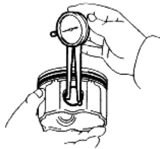
Fig. 416: Measuring Piston Pin Bore Diameter
