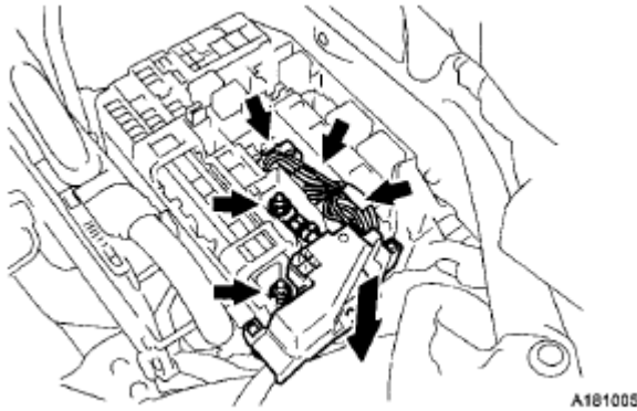
Fig. 226: Locating Wire Harness With Nuts
