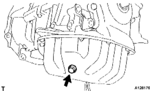
Fig. 253: Locating Oil Pan Drain Plug Courtesy of TOYOTA MOTOR SALES, U.S.A., INC.
