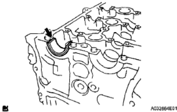
Fig. 315: Identifying No. 2 Camshaft Bearing Installation Position Courtesy of TOYOTA MOTOR SALES, U.S.A., INC.
