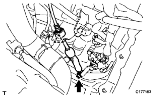
Fig. 183: Locating Control Cable Assembly Nuts Courtesy of TOYOTA MOTOR SALES, U.S.A., INC.
