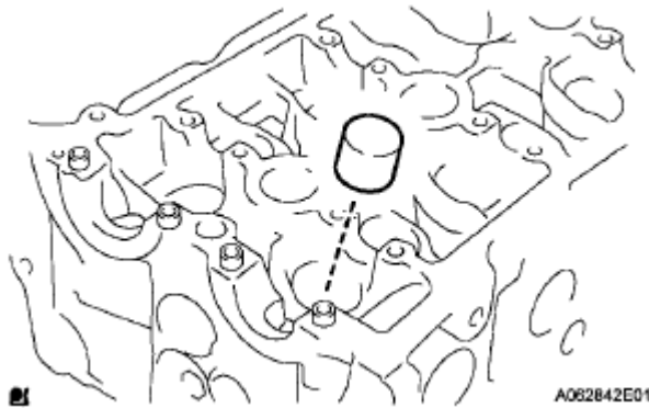
Fig. 326: Identifying Valve Lifters
