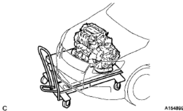
Fig. 194: Setting Engine Assembly With Transaxle On Engine Lifter Courtesy of TOYOTA MOTOR SALES, U.S.A., INC.
