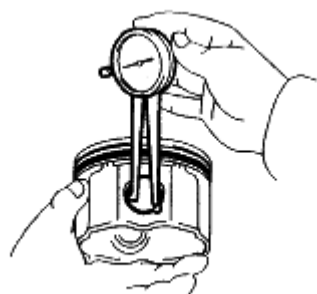
Fig. 403: Measuring Piston Pin Bore Diameter
