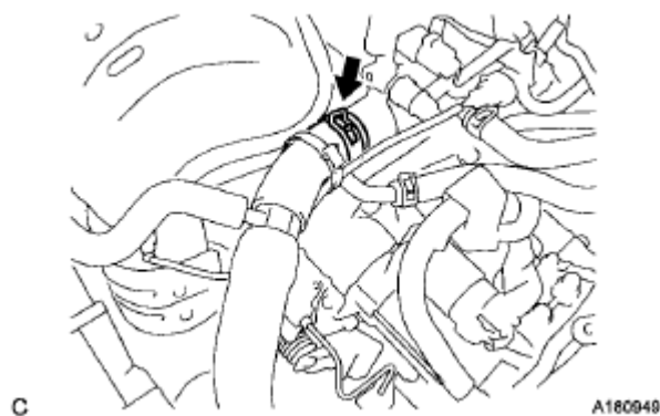
Fig. 167: Locating No. 1 Radiator Hose
