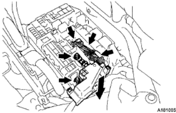
Fig. 213: Locating Wire Harness With Nuts Courtesy of TOYOTA MOTOR SALES, U.S.A., INC.
