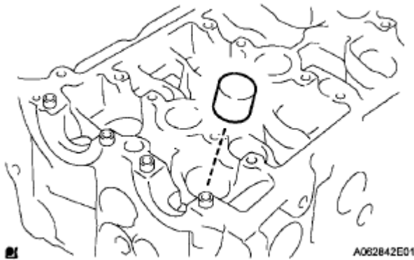
Fig. 326: Identifying Valve Lifters
