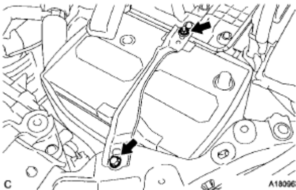
Fig. 216: Locating Battery Clamp With Bolt And Nut
