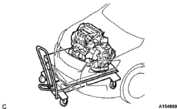
Fig. 179: Identifying Engine Assembly With Transaxle On Engine Lifter Courtesy of TOYOTA MOTOR SALES, U.S.A., INC.
