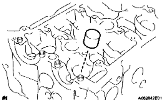
Fig. 373: Identifying Valve Lifter
