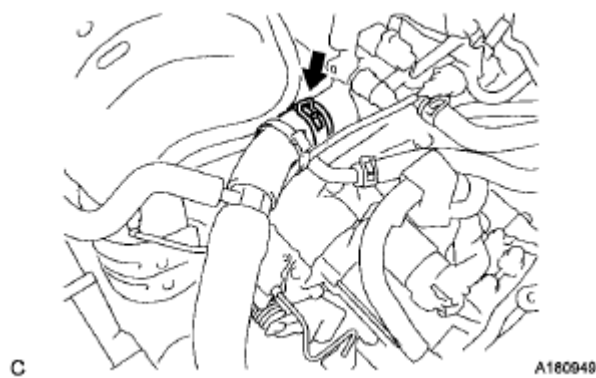
Fig. 167: Locating No. 1 Radiator Hose
