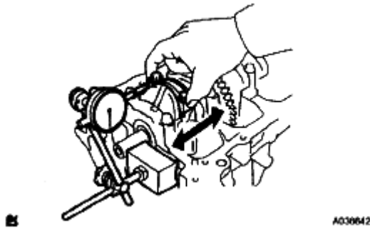
Fig. 390: Measuring Thrust Clearance
