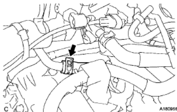
Fig. 206: Locating Outlet Heater Water Hose With Clamp Courtesy of TOYOTA MOTOR SALES, U.S.A., INC.
