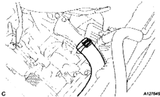
Fig. 315: Identifying Radiator Hose Outlet And Clamps Courtesy of TOYOTA MOTOR SALES, U.S.A., INC.
