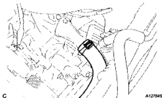
Fig. 232: Identifying Heater Inlet Water Hose Courtesy of TOYOTA MOTOR SALES, U.S.A., INC.
