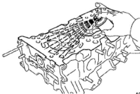
Fig. 402: Identifying Combustion Chamber, Intake Ports, Exhaust Ports And Cylinder Block Surface For Cracks Courtesy of TOYOTA MOTOR SALES, U.S.A., INC.
