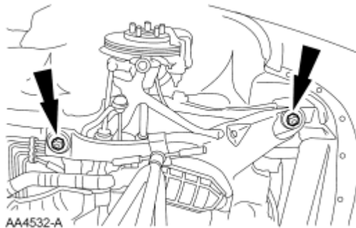
Fig. 29: Right Subframe Bolts Courtesy of FORD MOTOR CO.
