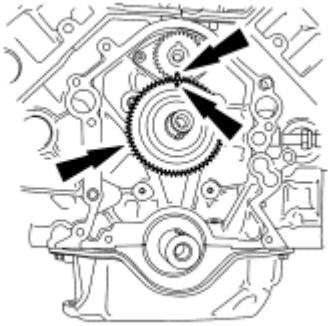
Fig. 317: Installing Engine Balance Shaft Drive Gear Courtesy of FORD MOTOR CO.
