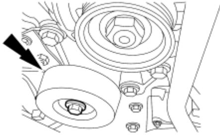
Fig. 211: Locating Accessory Drive Belt Idler Pulley Courtesy of FORD MOTOR CO.
