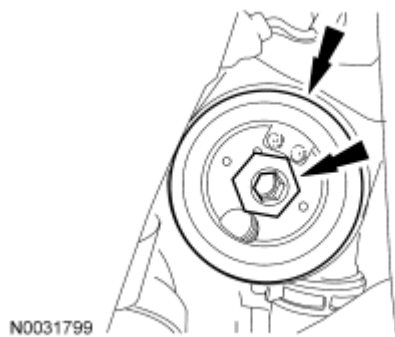
Fig. 257: Locating Oil Cooler/Tube Assembly & Bolt Courtesy of FORD MOTOR CO.
