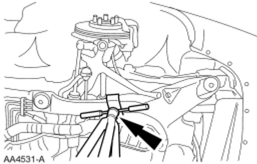
Fig. 28: Safety Stand Under Right Side Of Subframe Courtesy of FORD MOTOR CO.
