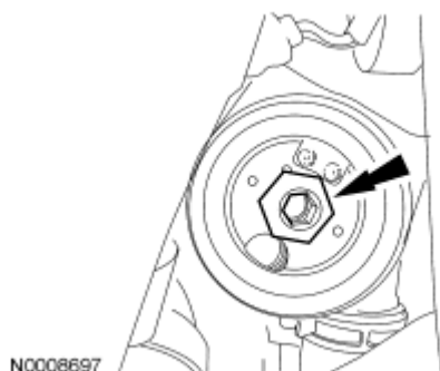
Fig. 115: Locating Oil Cooler Mounting Bolt Courtesy of FORD MOTOR CO.
