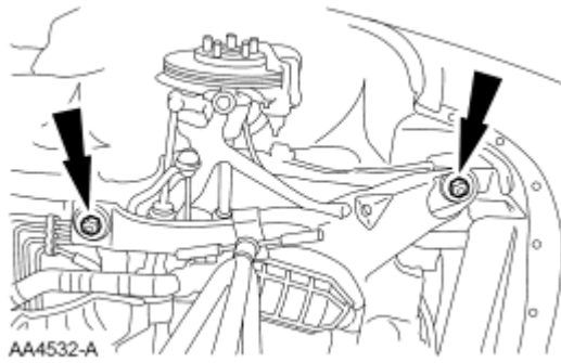
Fig. 50: Right Subframe Bolts Courtesy of FORD MOTOR CO.
