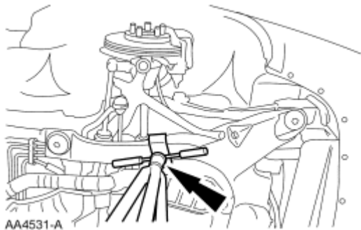
Fig. 46: Safety Stand Under Right Side Of Subframe Courtesy of FORD MOTOR CO.
