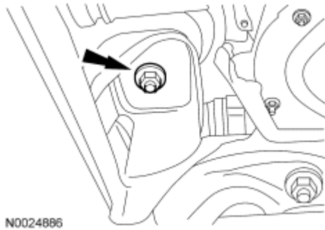
Fig. 175: Locating Lower Engine Mount Nuts Courtesy of FORD MOTOR CO.
