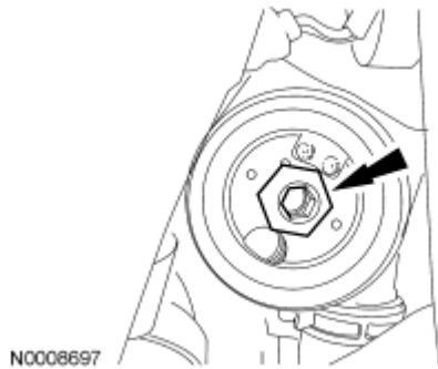
Fig. 116: Locating Oil Cooler Mounting Bolt Courtesy of FORD MOTOR CO.
