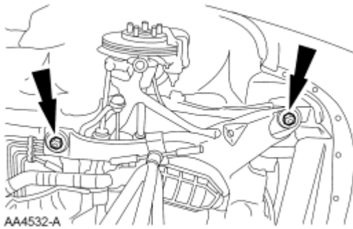
Fig. 34: Right Subframe Bolts Courtesy of FORD MOTOR CO.
