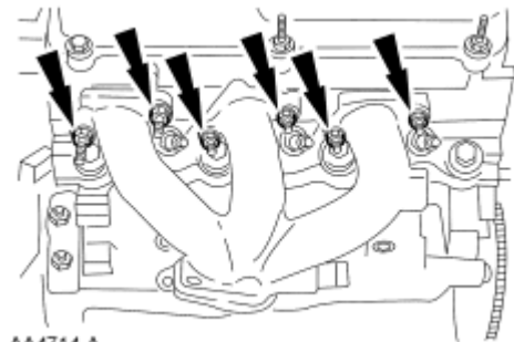
Fig. 353: Locating LH Exhaust Manifold Nuts Courtesy of FORD MOTOR CO.
