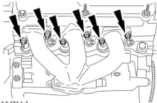
Fig. 258: Locating LH Exhaust Manifold Nuts Courtesy of FORD MOTOR CO.
