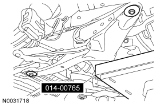
Fig. 193: Positioning Special Tool (014-00765)
