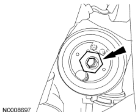
Fig. 126: Locating Oil Cooler Mounting Bolt Courtesy of FORD MOTOR CO.
