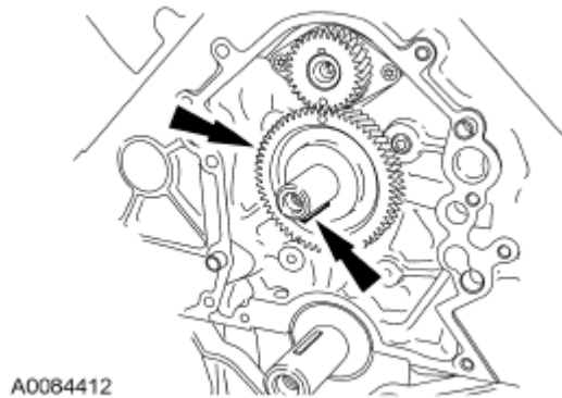
Fig. 280: Locating Engine Balance Shaft Drive Gear And Camshaft Key Courtesy of FORD MOTOR CO.
