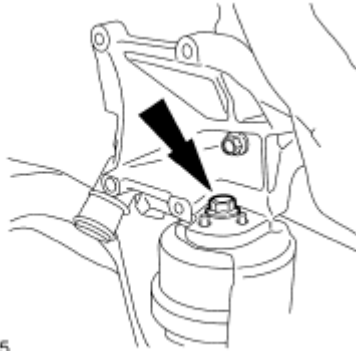
Fig. 417: Locating LH Engine Mount Bolt Courtesy of FORD MOTOR CO.
