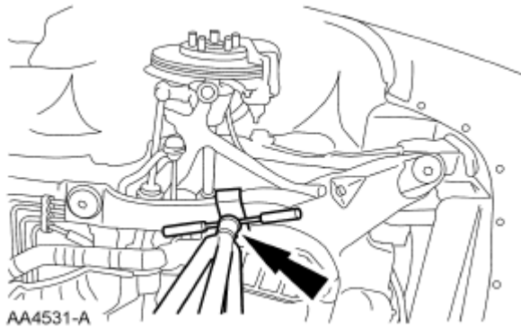
Fig. 28: Locating Safety Stand Under RH Side Of Subframe Courtesy of FORD MOTOR CO.
