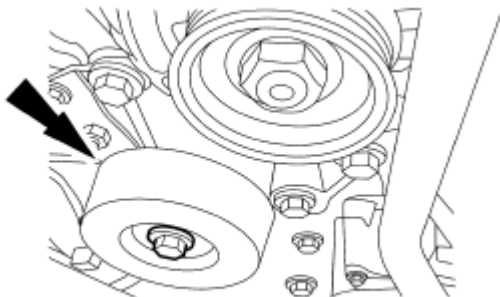
Fig. 221: Locating Accessory Drive Belt Idler Pulley Courtesy of FORD MOTOR CO.
