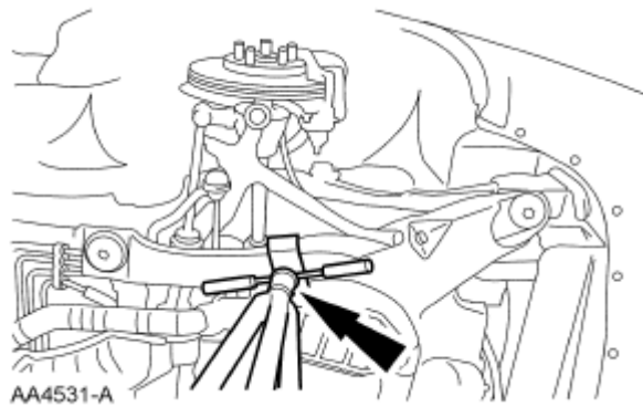
Fig. 46: Locating Safety Stand Under RH Side Of Subframe Courtesy of FORD MOTOR CO.
