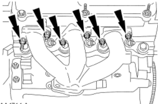
Fig. 364: Locating LH Exhaust Manifold Nuts Courtesy of FORD MOTOR CO.
