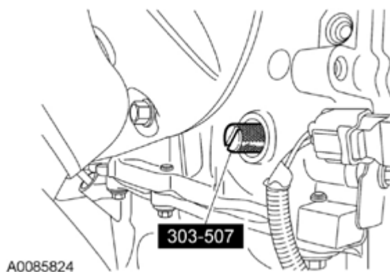
Fig. 487: Identifying Crankshaft TDC Timing Peg
