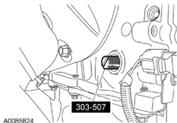
Fig. 479: Identifying Crankshaft TDC Timing Peg Courtesy of FORD MOTOR CO.
