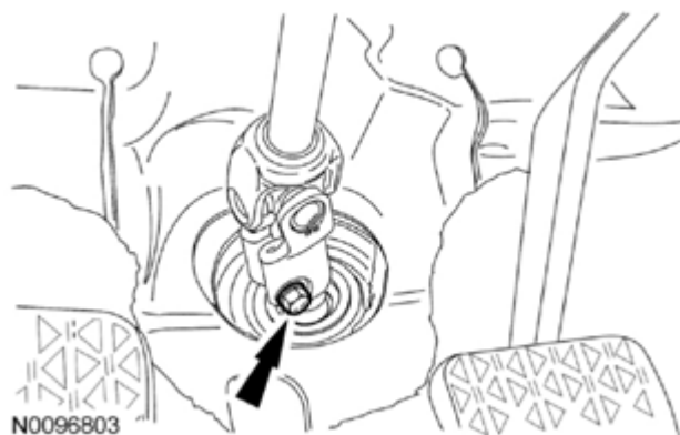
Fig. 651: Locating Steering Column Shaft Bolt Courtesy of FORD MOTOR CO.
