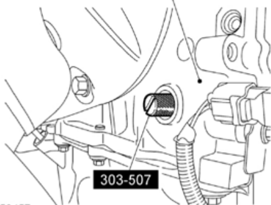
Fig. 366: Remove/Install Crankshaft TDC Timing Peg Courtesy of FORD MOTOR CO.
