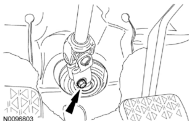
Fig. 593: Locating Steering Column Shaft Bolt Courtesy of FORD MOTOR CO.
