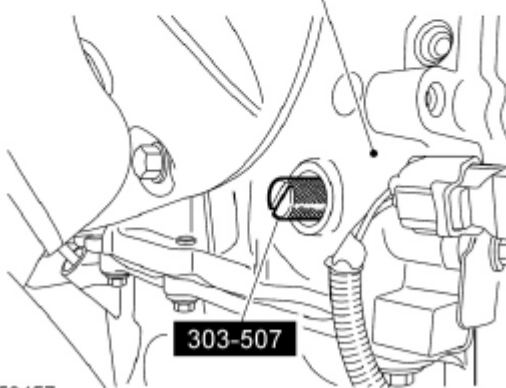
Fig. 4: Remove/Install Crankshaft TDC Timing Peg Courtesy of FORD MOTOR CO.
