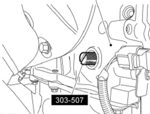
Fig. 122: Remove/Install Crankshaft TDC Timing Peg Courtesy of FORD MOTOR CO.
