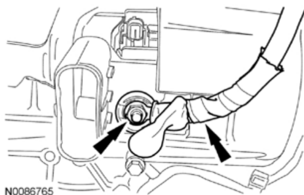
Fig. 311: Locating Nut And Generator B+ Wiring Harness Courtesy of FORD MOTOR CO.
