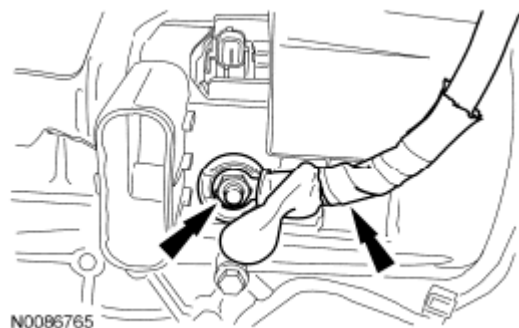
Fig. 249: Locating Nut & Generator B+ Wiring Harness Courtesy of FORD MOTOR CO.
