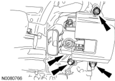
Fig. 522: Locating Nuts, Bolt & Generator Courtesy of FORD MOTOR CO.
