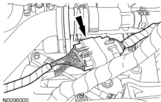
Fig. 598: Locating Engine Wiring Harness Electrical Connector Courtesy of FORD MOTOR CO.
