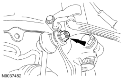
Fig. 638: Locating Sway Bar Links & Nuts Courtesy of FORD MOTOR CO.
