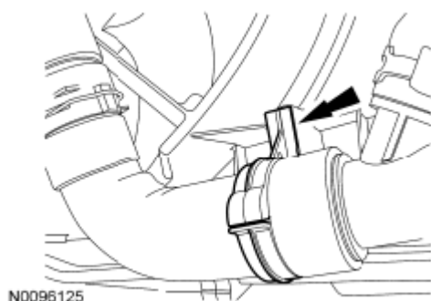
Fig. 297: Locating Lower Radiator Hose Pin-Type Retainer Courtesy of FORD MOTOR CO.
