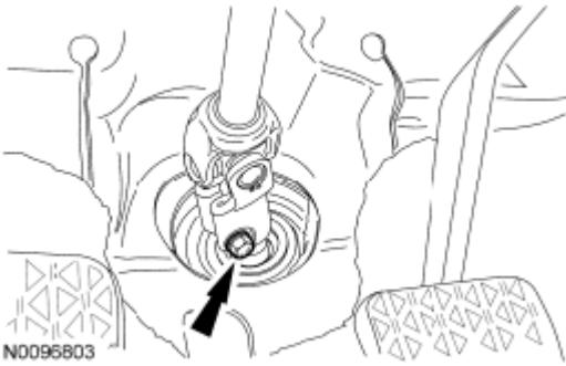
Fig. 198: Locating Steering Column Shaft Bolt Courtesy of FORD MOTOR CO.
