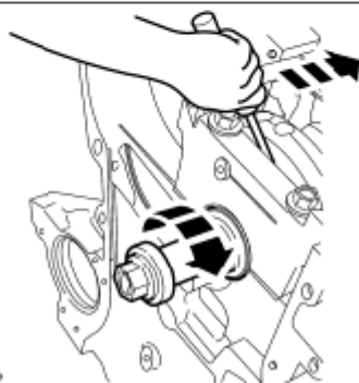
Fig. 16: Measuring Gear Backlash Courtesy of FORD MOTOR CO.
