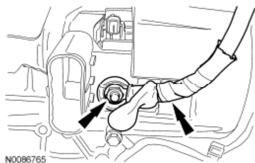
Fig. 544: Locating Generator B+ Wiring Harness & Nut Courtesy of FORD MOTOR CO.
