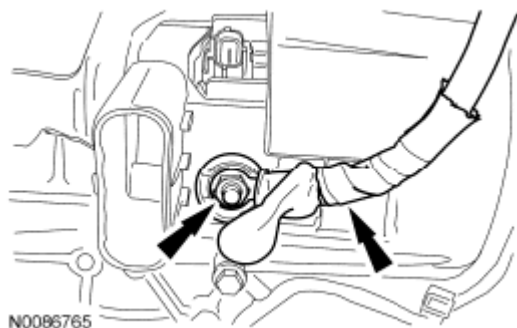
Fig. 311: Locating Nut & Generator Wiring Harness Courtesy of FORD MOTOR CO.
