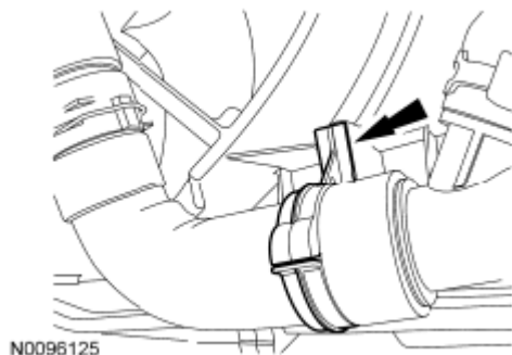
Fig. 615: Locating Lower Radiator Hose Pin-Type Retainer Courtesy of FORD MOTOR CO.
