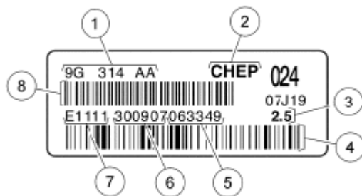
Fig. 1: Identifying Engine Code Information Label Courtesy of FORD MOTOR CO.
