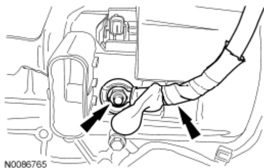
Fig. 602: Locating Generator B+ Wiring Harness & Nut Courtesy of FORD MOTOR CO.
