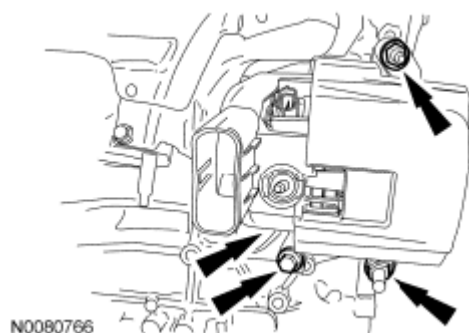
Fig. 330: Locating Nuts, Bolt & Generator Courtesy of FORD MOTOR CO.
