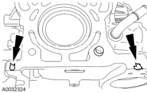
Fig. 164: Locating Silicone Gasket & Sealant Application Points Courtesy of FORD MOTOR CO.
