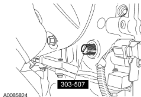
Fig. 38: Removing Crankshaft TDC Timing Peg Courtesy of FORD MOTOR CO.
