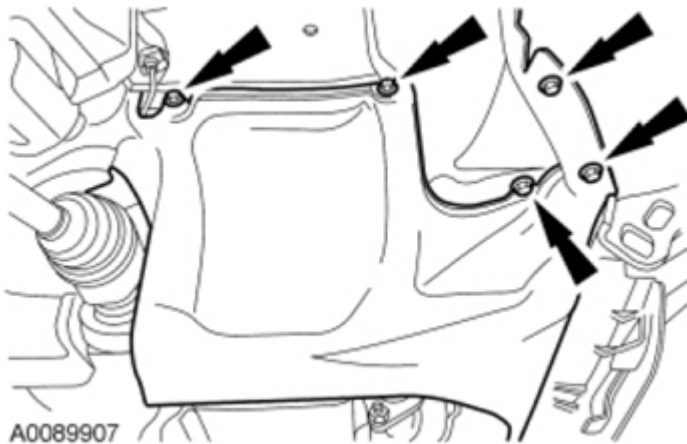
Fig. 160: Locating RH Splash Shield Bolts Courtesy of FORD MOTOR CO.
