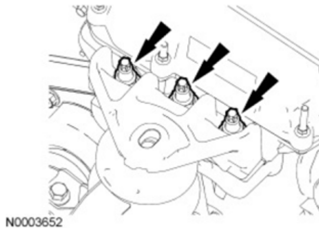
Fig. 560: Locating Engine Mount Bracket Nuts Courtesy of FORD MOTOR CO.
