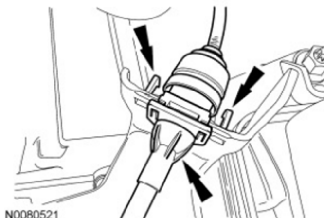
Fig. 199: View Of Transmission Shift Cable Tabs Courtesy of FORD MOTOR CO.
