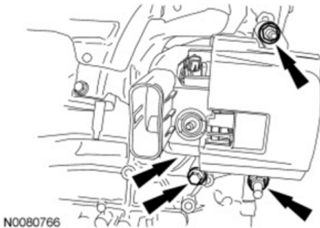
Fig. 282: Locating Generator With Fasteners Courtesy of FORD MOTOR CO.
