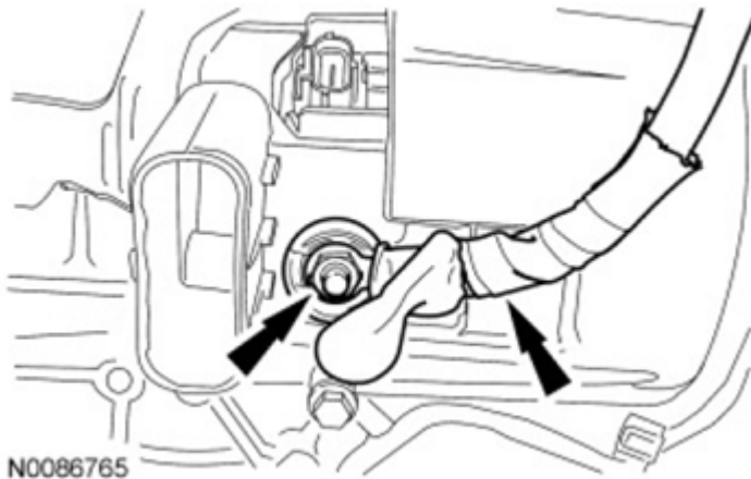
Fig. 281: Locating Generator Wiring Harness And Nut Courtesy of FORD MOTOR CO.
