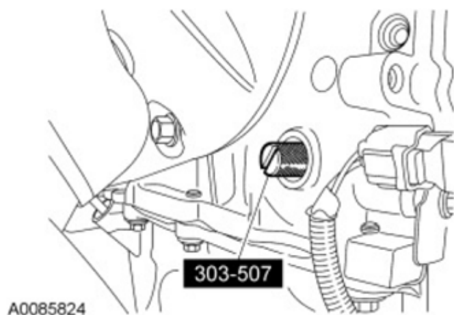
Fig. 134: View Of Crankshaft TDC Timing Peg Courtesy of FORD MOTOR CO.
