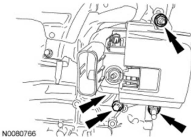
Fig. 490: Locating Generator With Fasteners Courtesy of FORD MOTOR CO.
