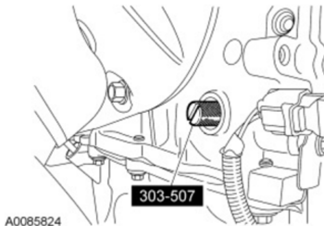
Fig. 435: View Of Crankshaft TDC Timing Peg Courtesy of FORD MOTOR CO.
