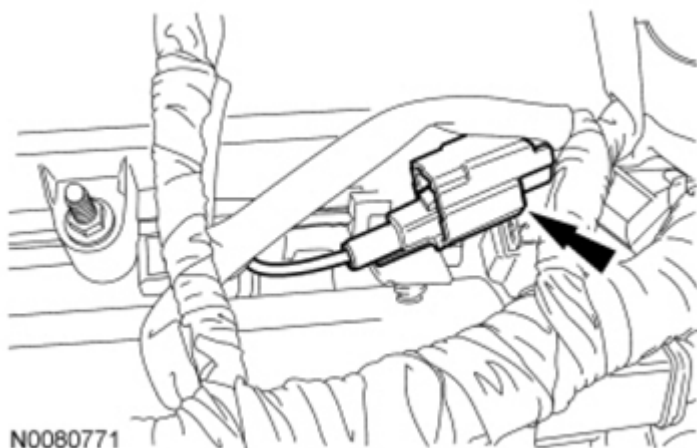
Fig. 465: Locating Radio Capacitor Electrical Connector Courtesy of FORD MOTOR CO.
