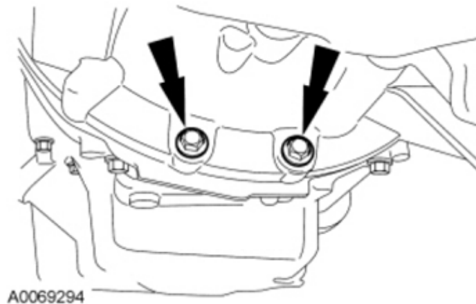
Fig. 264: Locating Transaxle-To-Engine Bolts Courtesy of FORD MOTOR CO.
