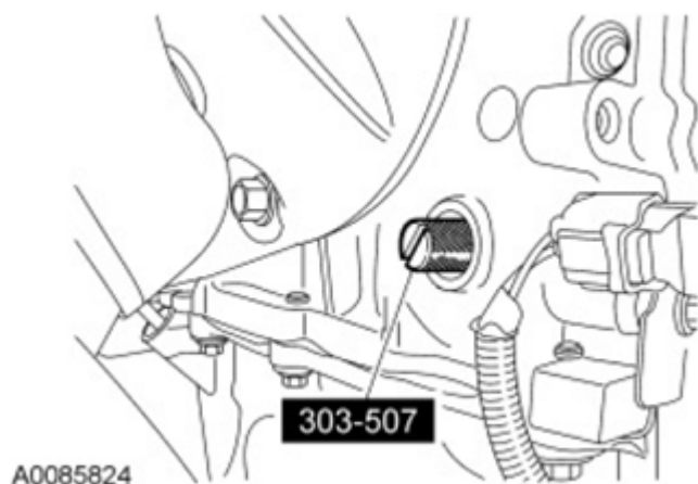
Fig. 445: View Of Crankshaft TDC Timing Peg Courtesy of FORD MOTOR CO.
