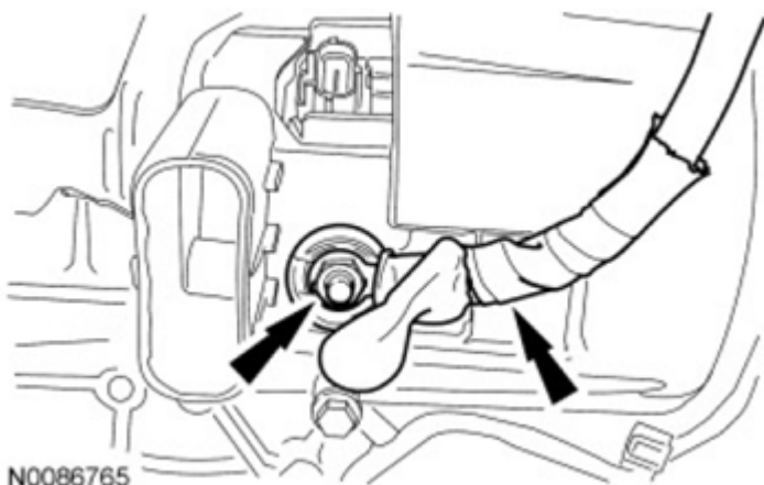
Fig. 491: Locating Generator Wiring Harness And Nut Courtesy of FORD MOTOR CO.
