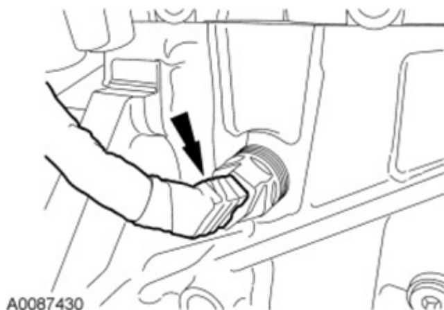
Fig. 533: Locating Block Heater Electrical Connector Courtesy of FORD MOTOR CO.
