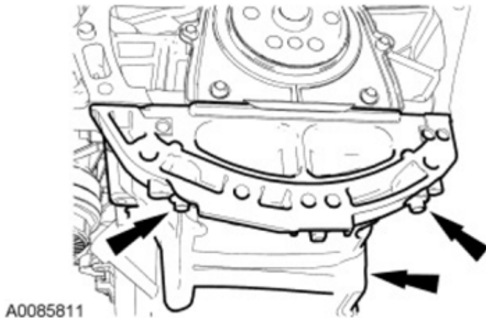
Fig. 53: Locating Oil Pan Bolts Courtesy of FORD MOTOR CO.
