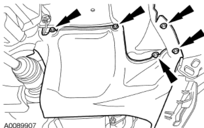
Fig. 160: Identifying RH Splash Shield And Retainers Courtesy of FORD MOTOR CO.
