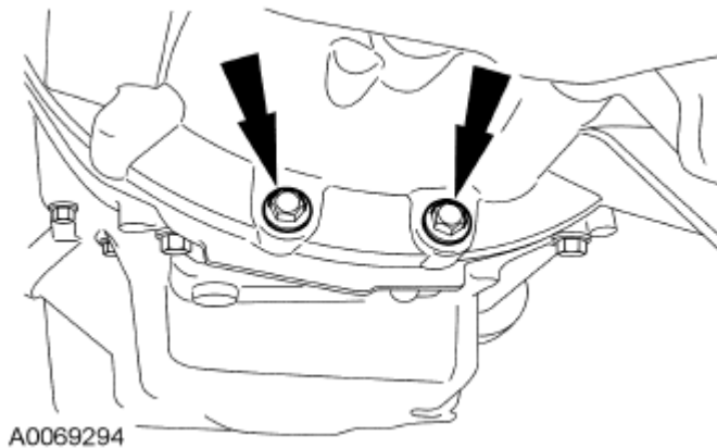
Fig. 564: Locating Transaxle-To-Engine Bolts Courtesy of FORD MOTOR CO.
