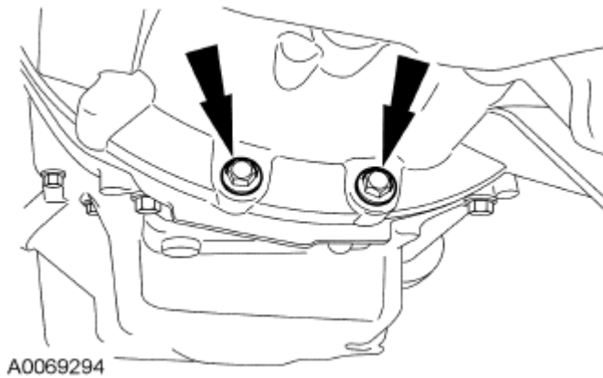
Fig. 519: Locating Transaxle-To-Engine Bolts Courtesy of FORD MOTOR CO.
