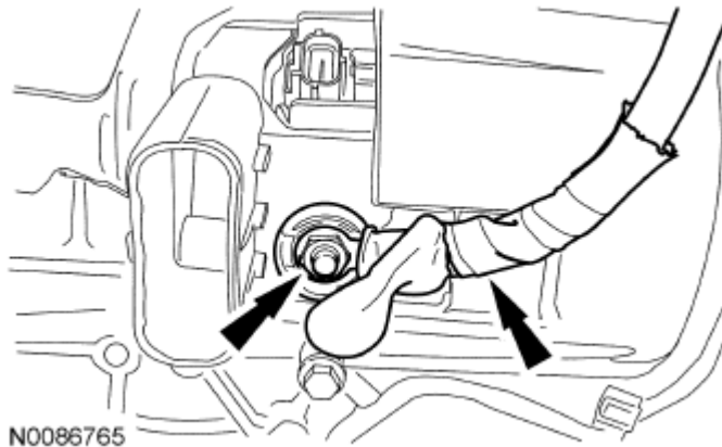
Fig. 491: Locating Nut And Generator Wiring Harness Courtesy of FORD MOTOR CO.
