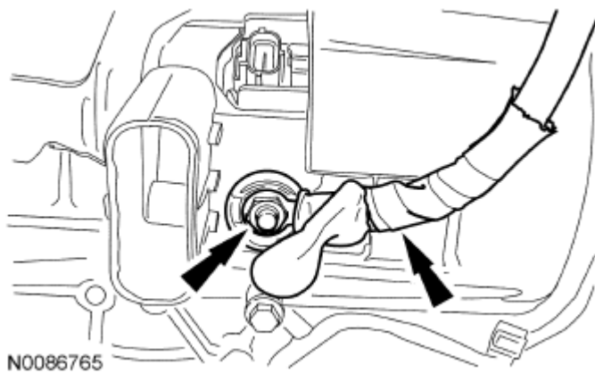
Fig. 281: Locating Nut And Generator Wiring Harness Courtesy of FORD MOTOR CO.
