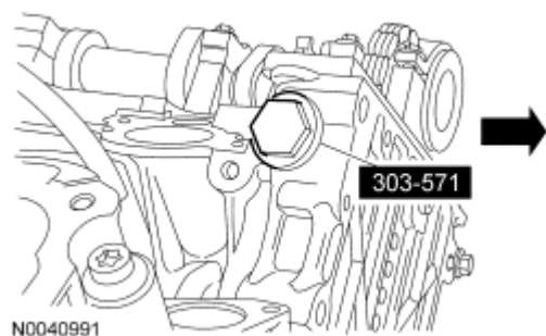
Fig. 352: Identifying Special Tool (303-571) Courtesy of FORD MOTOR CO.
