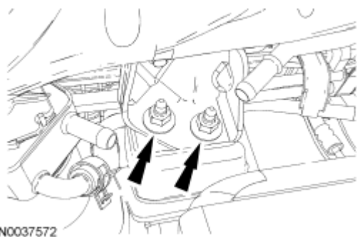
Fig. 161: Locating RH Engine Support Insulator Nuts Courtesy of FORD MOTOR CO.
