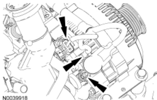
Fig. 172: Identifying Generator Electrical Connectors And Wire Harness Retainer Courtesy of FORD MOTOR CO.
