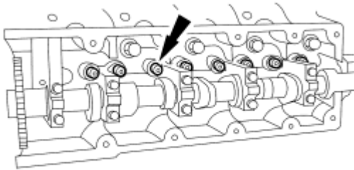
Fig. 263: Locating Hydraulic Lash Adjusters Courtesy of FORD MOTOR CO.
