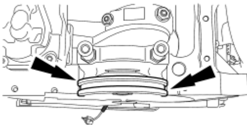
Fig. 108: Locating Sealant Position On Rear Main Bearing Cap Courtesy of FORD MOTOR CO.
