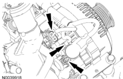
Fig. 393: Identifying Generator Electrical Connectors And Wire Harness Retainer Courtesy of FORD MOTOR CO.
