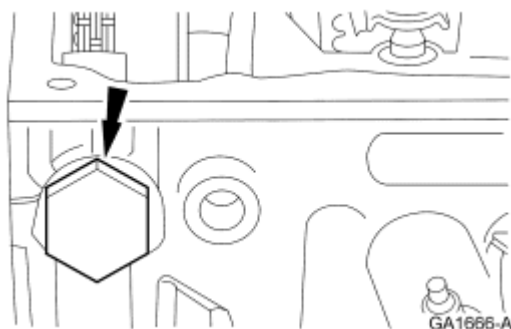
Fig. 349: Locating RH Hydraulic Chain Tensioner Courtesy of FORD MOTOR CO.
