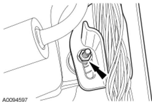
Fig. 216: Locating Wiring Conduit Nut Courtesy of FORD MOTOR CO.
