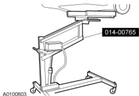
Fig. 148: Supporting Powertrain & Subframe Using Special Tool Courtesy of FORD MOTOR CO.
