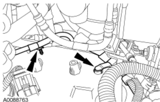
Fig. 156: Locating Wire Harness Retainers At Transaxle Courtesy of FORD MOTOR CO.
