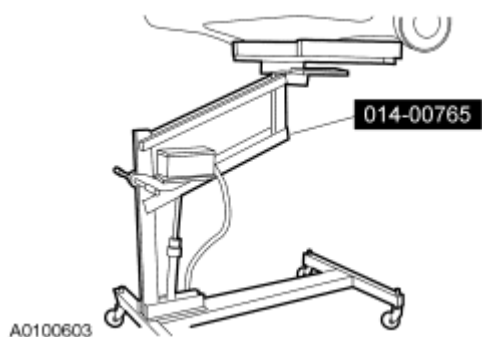
Fig. 144: Supporting Powertrain & Subframe Using Special Tool Courtesy of FORD MOTOR CO.
