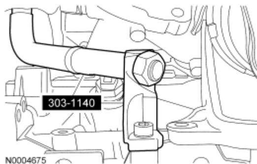
Fig. 372: Identifying Upper Half Of Lifting Hook Courtesy of FORD MOTOR CO.
