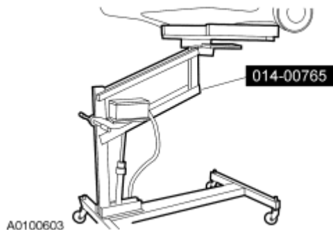
Fig. 411: Supporting Powertrain & Subframe Using Special Tool Courtesy of FORD MOTOR CO.
