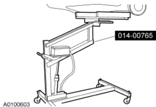
Fig. 141: Lowering Powertrain & Subframe From Vehicle Using Special Tool Courtesy of FORD MOTOR CO.
