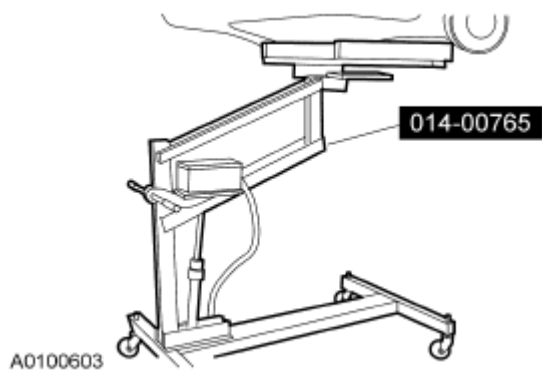
Fig. 145: Supporting Powertrain & Subframe Using Special Tool Courtesy of FORD MOTOR CO.
