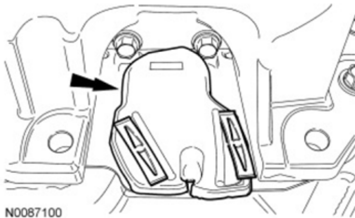
Fig. 202: Locating Access Cover Courtesy of FORD MOTOR CO.
