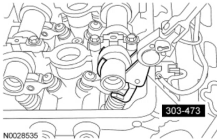
Fig. 118: Removing Roller Follower Using The Valve Spring Compressor Courtesy of FORD MOTOR CO.
