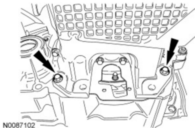
Fig. 204: Locating Oil Pan-To-Transaxle Bolts Courtesy of FORD MOTOR CO.
