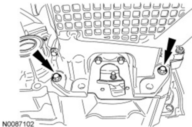
Fig. 475: Locating Oil Pan-To-Transaxle Bolts Courtesy of FORD MOTOR CO.
