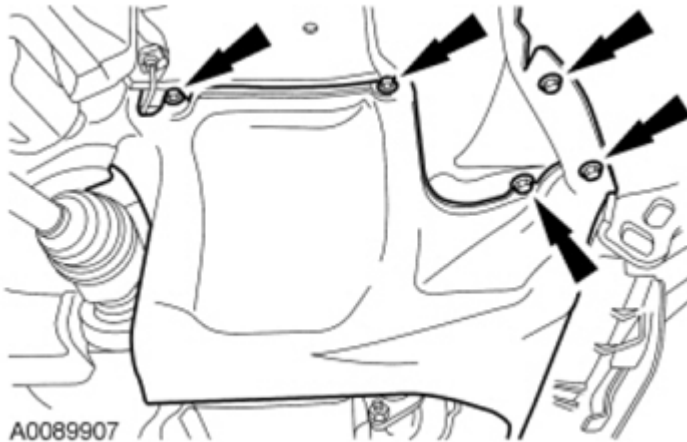
Fig. 66: Identifying RH Lower Splash Shield Bolts Courtesy of FORD MOTOR CO.
