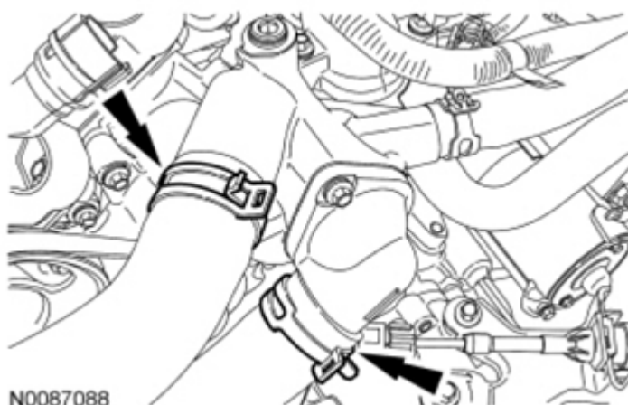
Fig. 188: Locating Upper And Lower Radiator Hoses Courtesy of FORD MOTOR CO.
