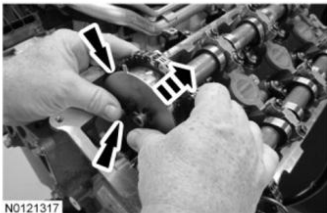
Fig. 73: Pressing LH Camshaft Phaser And Sprocket Bolt Towards The Rear Of The Engine Courtesy of FORD MOTOR CO.
