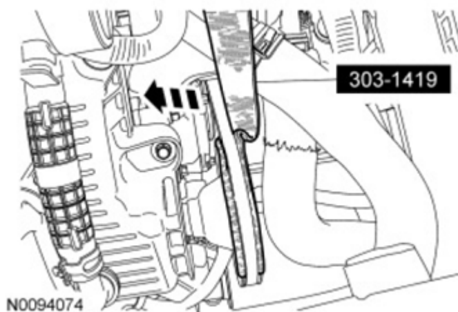
Fig. 273: Removing Coolant Pump Belt Using Stretchy Belt Remover Courtesy of FORD MOTOR CO.
