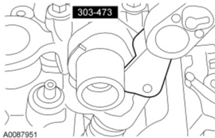
Fig. 122: Remove/Install Key, Retainer And The Valve Spring Using The Valve Spring Compressor Courtesy of FORD MOTOR CO.
