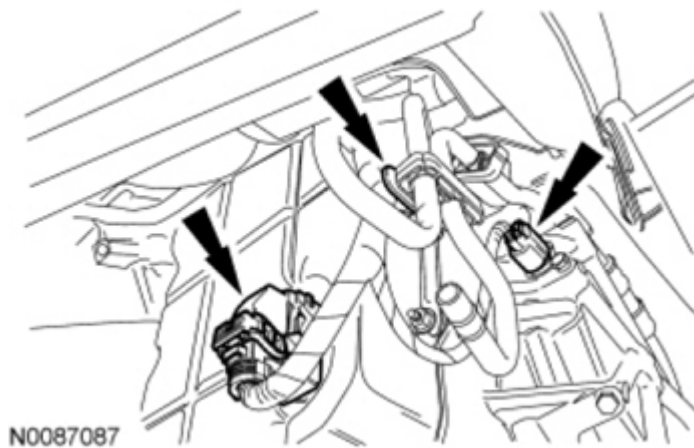
Fig. 493: Locating Transmission Electrical Connector And Wiring Retainer Courtesy of FORD MOTOR CO.
