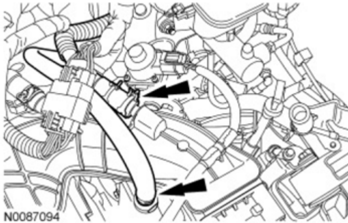
Fig. 486: Locating Evaporative Emission Canister Purge Valve Tube And Brake Booster Vacuum Tube
