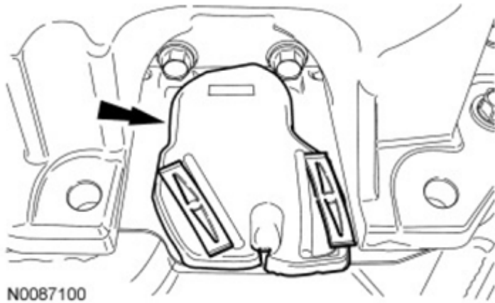
Fig. 478: Locating Access Cover Courtesy of FORD MOTOR CO.
