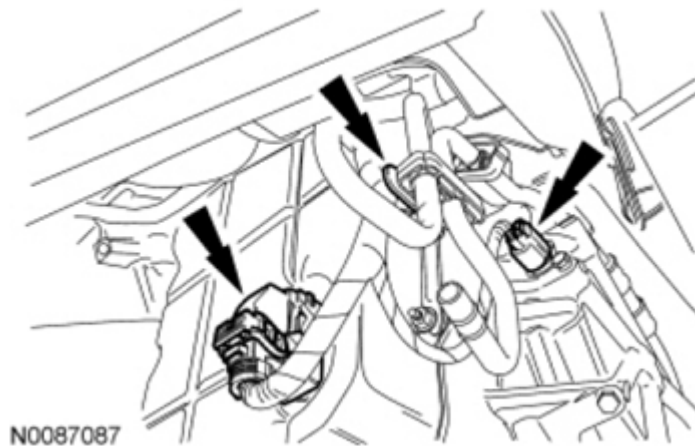
Fig. 187: Locating Transmission Electrical Connector And Wiring Retainer Courtesy of FORD MOTOR CO.
