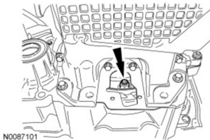
Fig. 203: Locating Torque Converter Nut Courtesy of FORD MOTOR CO.
