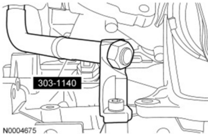
Fig. 225: Installing Upper Half Of Lifting Hook Courtesy of FORD MOTOR CO.
