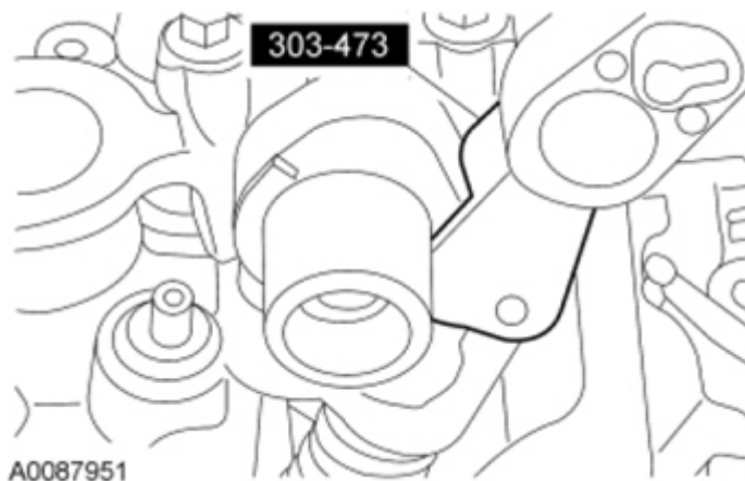
Fig. 119: Remove/Install Key, Retainer And The Valve Spring Using The Valve Spring Compressor Courtesy of FORD MOTOR CO.
