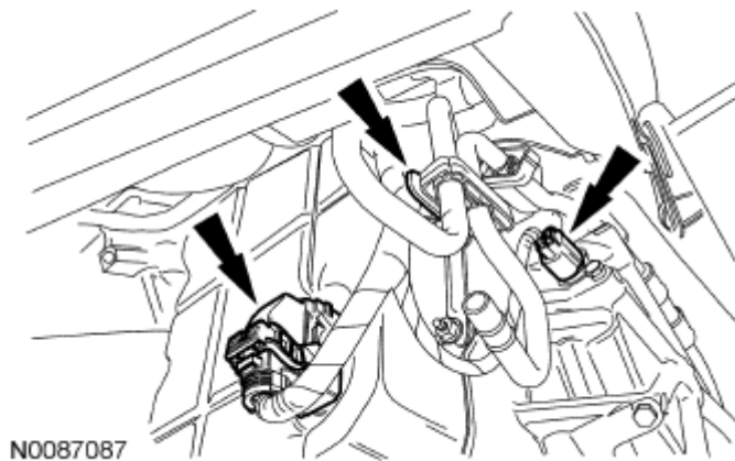
Fig. 440: Locating Transmission Electrical Connector Courtesy of FORD MOTOR CO.
