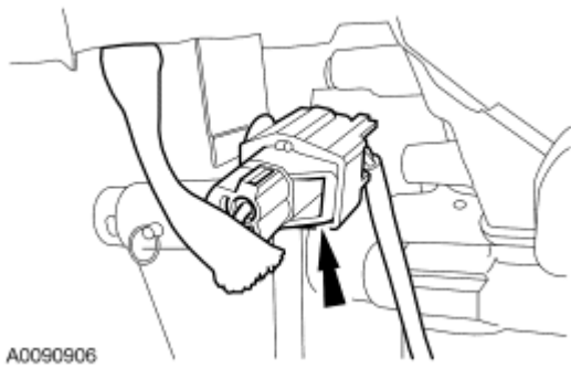
Fig. 162: Locating Knock Sensor (KS) Electrical Connector Courtesy of FORD MOTOR CO.
