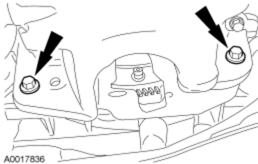
Fig. 342: Locating Oil Pan-To-Transaxle Bolts Courtesy of FORD MOTOR CO.
