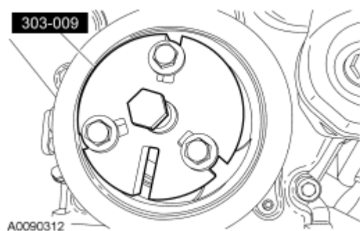
Fig. 202: Removing Crankshaft Pulley Using Special Tool (303-009) Courtesy of FORD MOTOR CO.
