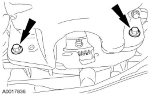
Fig. 140: Locating Oil Pan-To-Transaxle Bolts Courtesy of FORD MOTOR CO.
