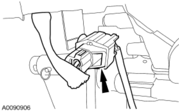
Fig. 327: Locating KS Electrical Connector Courtesy of FORD MOTOR CO.
