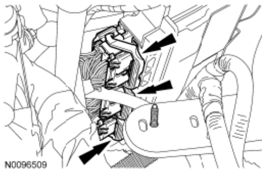
Fig. 158: Locating PCM Electrical Connectors Courtesy of FORD MOTOR CO.
