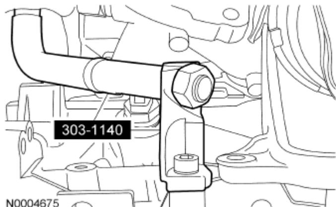
Fig. 194: Identifying Upper Half Of Lifting Hook Courtesy of FORD MOTOR CO.
