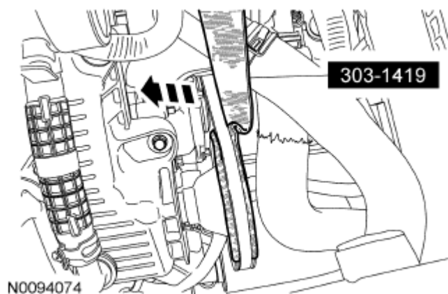
Fig. 240: Removing Coolant Pump Belt Courtesy of FORD MOTOR CO.
