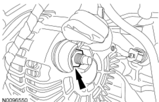
Fig. 412: Locating B+ Wire & Nut On Generator Courtesy of FORD MOTOR CO.
