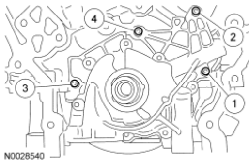
Fig. 113: Identifying Oil Pump Bolts In Tightening Sequence Courtesy of FORD MOTOR CO.
