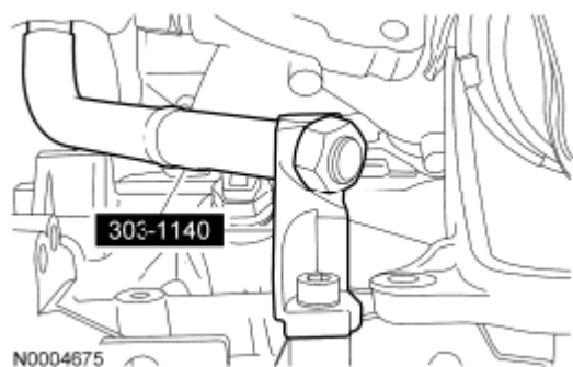
Fig. 416: Removing Nuts At Lift Links Courtesy of FORD MOTOR CO.
