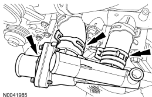
Fig. 283: Locating Clamps And Thermostat Housing Courtesy of FORD MOTOR CO.
