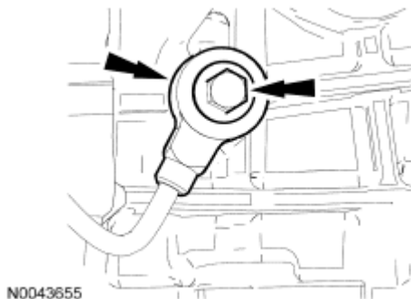
Fig. 395: Locating Knock Sensor (KS) And Bolt Courtesy of FORD MOTOR CO.
