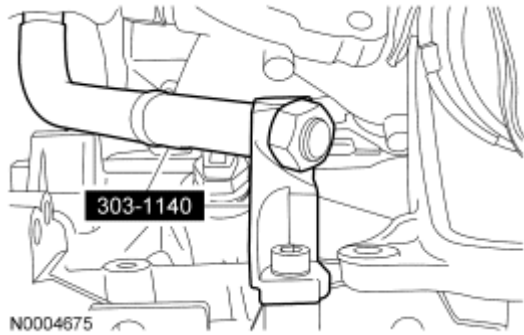
Fig. 217: Identifying Upper Half Of Lifting Hook Courtesy of FORD MOTOR CO.
