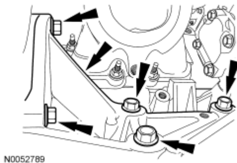
Fig. 193: Identifying PTU Support Bracket Bolts Courtesy of FORD MOTOR CO.
