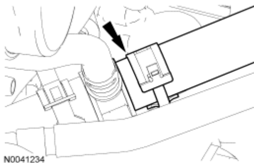
Fig. 164: Locating Heater Hose Inline Connection Courtesy of FORD MOTOR CO.
