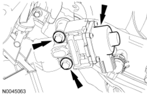
Fig. 480: Locating EGR Valve And Bolts Courtesy of FORD MOTOR CO.
