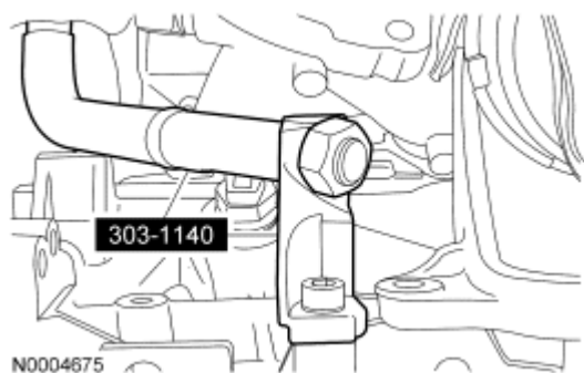
Fig. 449: Identifying Upper Half Of Lifting Hook Courtesy of FORD MOTOR CO.
