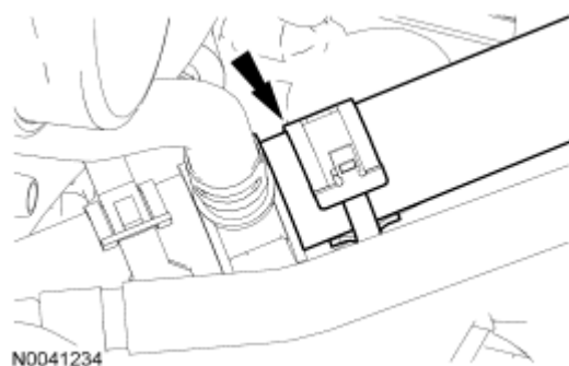
Fig. 525: Locating Heater Hose Inline Connection Courtesy of FORD MOTOR CO.
