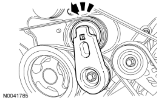
Fig. 421: Rotating Accessory Drive Belt Tensioner Counterclockwise Courtesy of FORD MOTOR CO.
