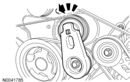
Fig. 266: Rotating Accessory Drive Belt Tensioner Counterclockwise Courtesy of FORD MOTOR CO.
