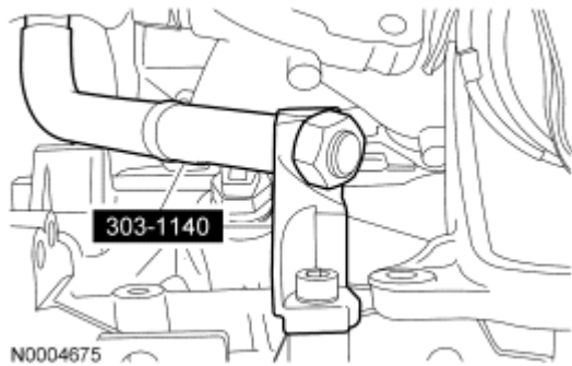
Fig. 419: Identifying Upper Half Of Lifting Hook Courtesy of FORD MOTOR CO.
