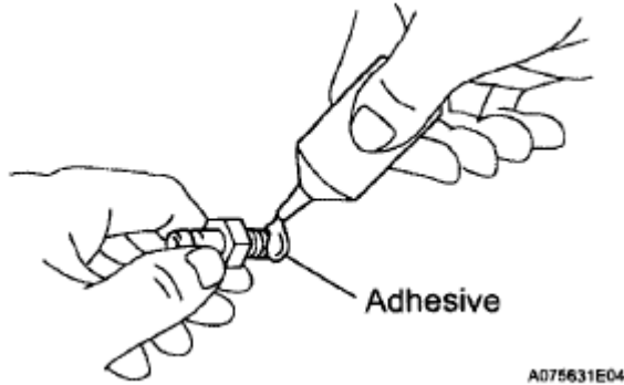
Fig. 570: Applying Adhesive To Threads Of Bolt End Courtesy of TOYOTA MOTOR SALES, U.S.A., INC.
