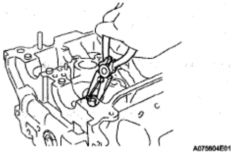
Fig. 432: Removing Valve Stem Oil O Seal Or Ring Courtesy of TOYOTA MOTOR SALES, U.S.A., INC.
