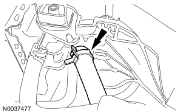
Fig. 235: Locating Power Steering Cooler Tube Courtesy of FORD MOTOR CO.
