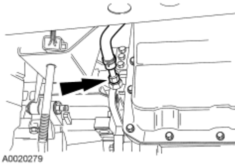
Fig. 455: Locating Transmission Fluid Cooler Tube Courtesy of FORD MOTOR CO.
