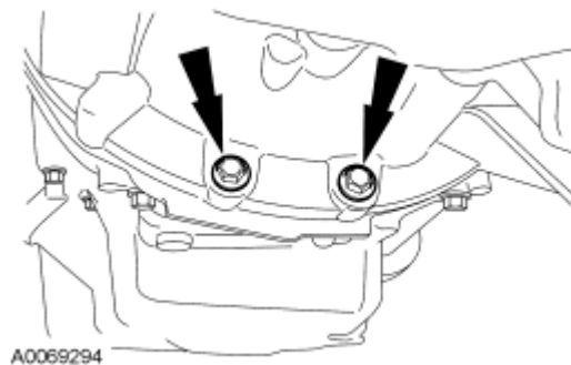
Fig. 177: Locating Lower Bellhousing Bolts Courtesy of FORD MOTOR CO.
