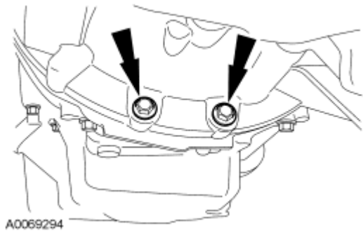
Fig. 477: Locating Lower Bellhousing Bolts Courtesy of FORD MOTOR CO.
