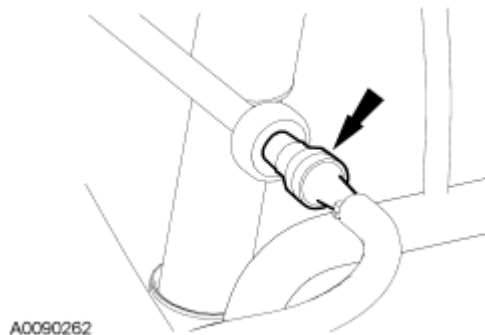
Fig. 165: Vacuum Reservoir Tube Courtesy of FORD MOTOR CO.
