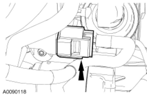
Fig. 392: Locating Temperature Manifold Absolute Pressure (TMAP) Electrical Connector Courtesy of FORD MOTOR CO.
