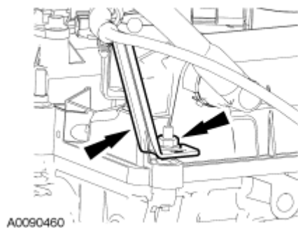
Fig. 211: Accelerator Control Cable Bracket & Nut Courtesy of FORD MOTOR CO.
