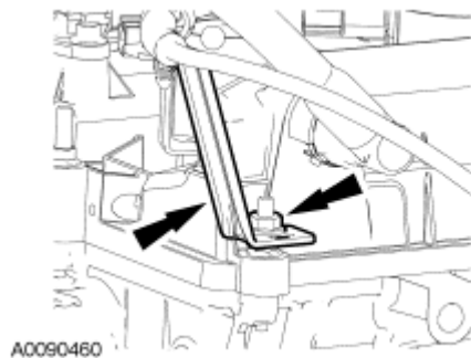
Fig. 443: Accelerator Control Cable Bracket & Nut Courtesy of FORD MOTOR CO.
