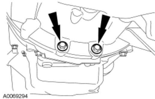
Fig. 227: Locating Lower Bellhousing Bolts Courtesy of FORD MOTOR CO.
