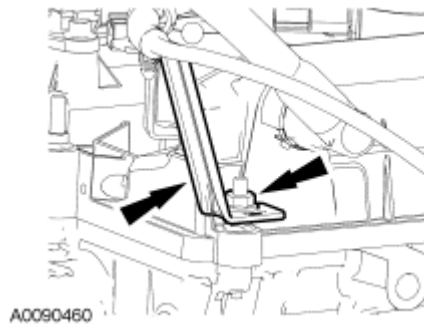
Fig. 161: Accelerator Control Cable Bracket & Nut Courtesy of FORD MOTOR CO.
