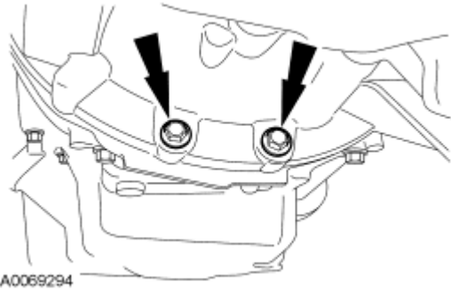
Fig. 426: Locating Lower Bellhousing Bolts Courtesy of FORD MOTOR CO.
