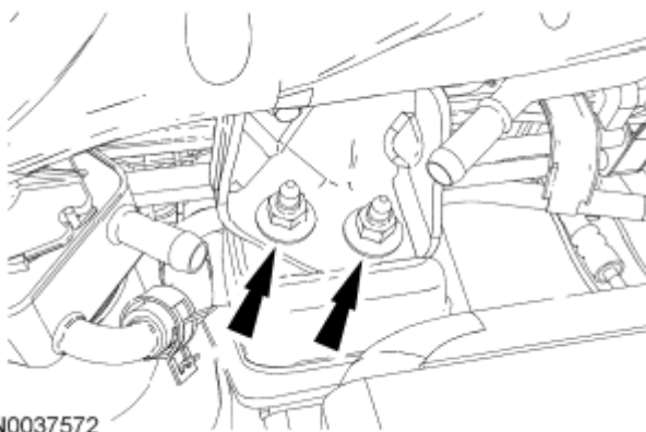
Fig. 164: Locating RH Engine Support Insulator Nuts Courtesy of FORD MOTOR CO.
