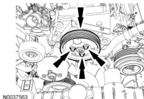
Fig. 147: Locating Power Steering Pump Pulley And Bolts Courtesy of FORD MOTOR CO.
