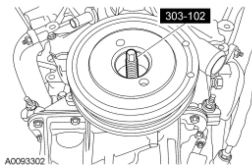
Fig. 337: Installing Crankshaft Pulley Using Special Tool Courtesy of FORD MOTOR CO.
