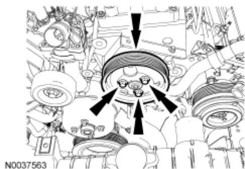
Fig. 423: Locating Power Steering Pump Pulley And Bolts Courtesy of FORD MOTOR CO.
