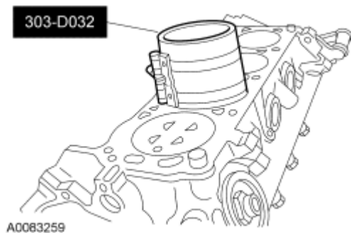
Fig. 284: Installing Piston Using Special Tool (303-D032) Courtesy of FORD MOTOR CO.
