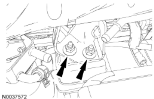
Fig. 405: Locating RH Engine Support Insulator Nuts Courtesy of FORD MOTOR CO.
