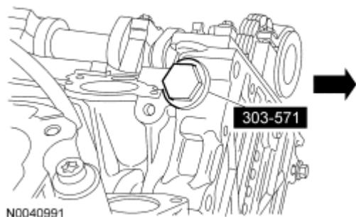
Fig. 23: Identifying Special Tool (303-571) Courtesy of FORD MOTOR CO.
