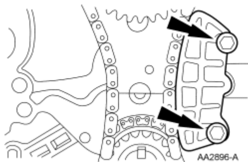
Fig. 244: Locating Chain Guide & Bolts Courtesy of FORD MOTOR CO.
