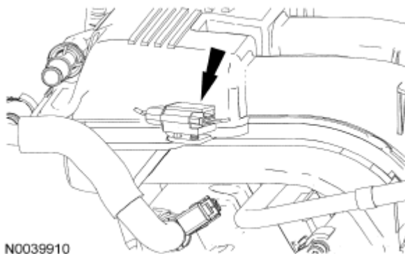
Fig. 463: Locating KS Electrical Connector
