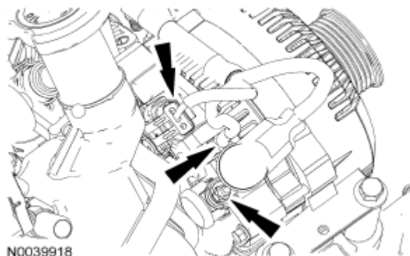
Fig. 475: Locating Generator Electrical Connections And Wire Harness Retainer Courtesy of FORD MOTOR CO.
