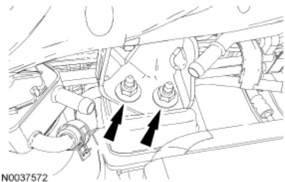
Fig. 232: Locating RH Engine Support Insulator Nuts Courtesy of FORD MOTOR CO.
