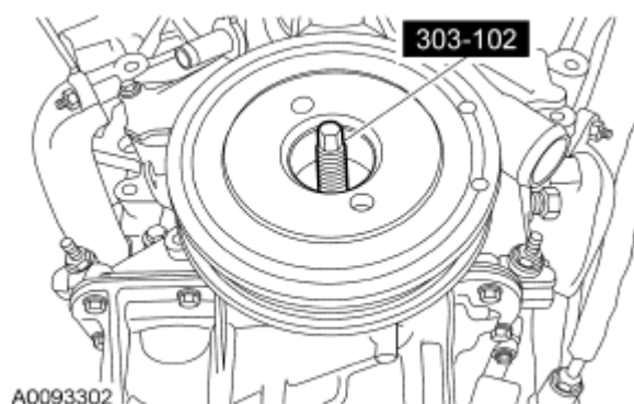
Fig. 418: Identifying Special Tool And Crankshaft Pulley Courtesy of FORD MOTOR CO.
