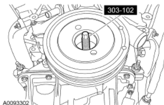
Fig. 42: Identifying Special Tool And Crankshaft Pulley. Courtesy of FORD MOTOR CO.
