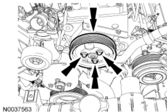
Fig. 218: Locating Power Steering Pump Pulley And Bolts Courtesy of FORD MOTOR CO.
