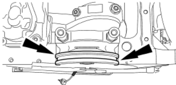
Fig. 169: Locating Rear Main Bearing Cap Courtesy of FORD MOTOR CO.
