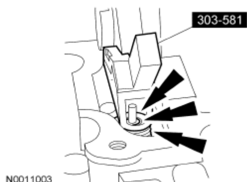
Fig. 343: Locating Special Tool, Valve Spring, Retainer And Retainer Keys Courtesy of FORD MOTOR CO.
