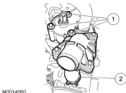
Fig. 443: Locating Bypass Hose Clamp And Bolts Courtesy of FORD MOTOR CO.
