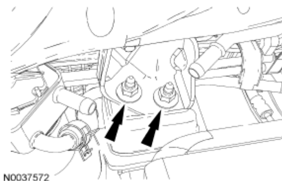
Fig. 487: Locating RH Engine Support Insulator Nuts Courtesy of FORD MOTOR CO.
