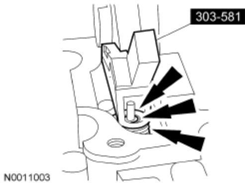
Fig. 337: Locating Special Tool, Valve Spring Retainer Keys, Valve Spring, Retainer And Valve Courtesy of FORD MOTOR CO.
