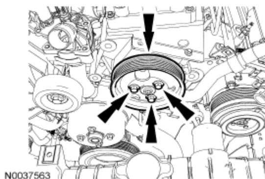
Fig. 505: Locating Power Steering Pump Pulley And Bolts Courtesy of FORD MOTOR CO.
