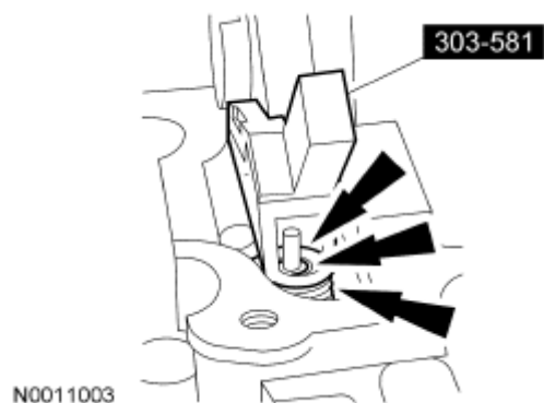
Fig. 150: Locating Special Tool, Valve Spring Retainer Keys, Valve Spring Retainers And Valve Springs
