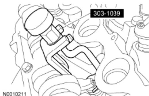
Fig. 179: Identifying Valve Spring Compressor Courtesy of FORD MOTOR CO.
