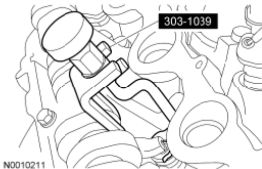
Fig. 131: Identifying Valve Spring Compressor Courtesy of FORD MOTOR CO.
