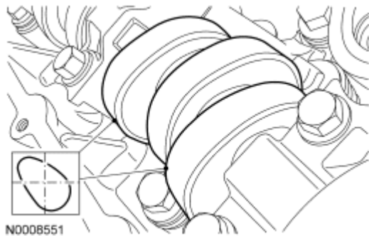
Fig. 111: Identifying Camshaft Lobe Position Courtesy of FORD MOTOR CO.
