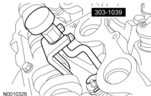
Fig. 139: Compressing Valve Spring With Special Tool Courtesy of FORD MOTOR CO.
