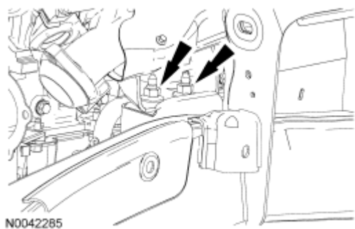
Fig. 200: Locating RH Engine Support Insulator Nuts Courtesy of FORD MOTOR CO.
