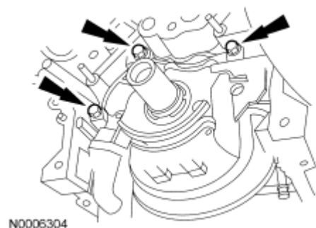
Fig. 162: Locating Oil Pump Bolts Courtesy of FORD MOTOR CO.
