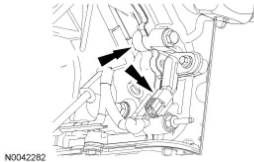
Fig. 205: Locating Crankshaft Position Sensor Electrical Connector And Wiring Harness Retainer Courtesy of FORD MOTOR CO.
