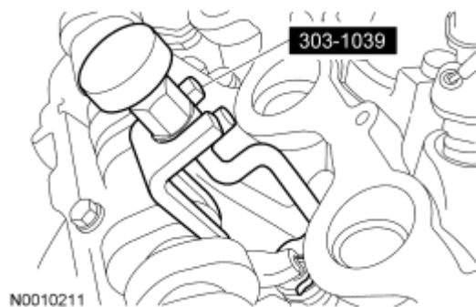
Fig. 113: Identifying Special Tool For Removing/Installing Camshaft Roller Followers
