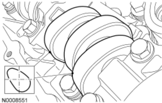
Fig. 233: Identifying Camshaft Lobe Position Courtesy of FORD MOTOR CO.
