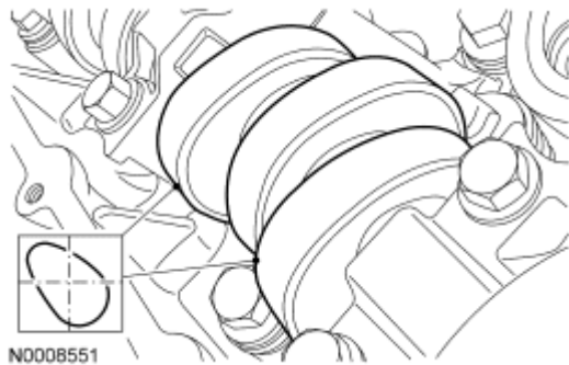
Fig. 308: Identifying Camshaft Lobe Position Courtesy of FORD MOTOR CO.
