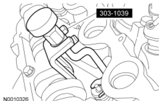
Fig. 144: Compressing Valve Spring With Special Tool Courtesy of FORD MOTOR CO.
