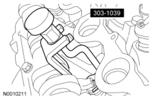
Fig. 136: Identifying Special Tool For Removing/Installing Camshaft Roller Followers Courtesy of FORD MOTOR CO.
