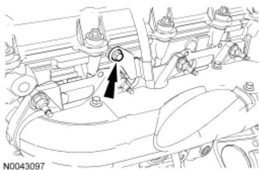
Fig. 526: Locating Oil Level Indicator Tube Bolt Courtesy of FORD MOTOR CO.
