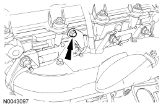
Fig. 222: Locating Oil Level Indicator Tube Bolt Courtesy of FORD MOTOR CO.
