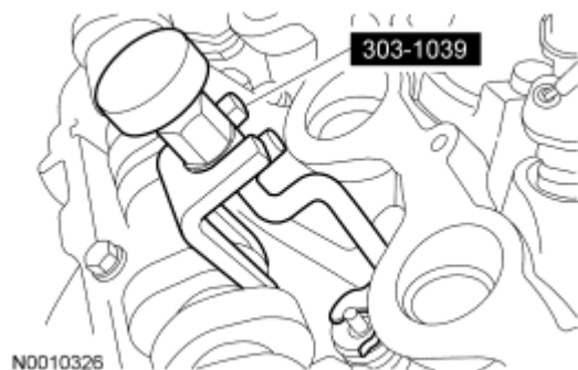
Fig. 142: Compressing Valve Spring With Special Tool Courtesy of FORD MOTOR CO.
