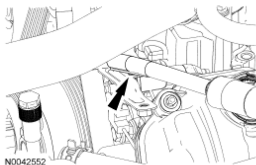
Fig. 177: Locating Wiring Harness Retainer From Cooling Fan Wiring Harness Bracket Courtesy of FORD MOTOR CO.
