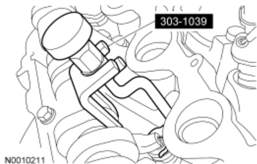
Fig. 141: Identifying Special Tool For Removing/Installing Camshaft Roller Followers Courtesy of FORD MOTOR CO.
