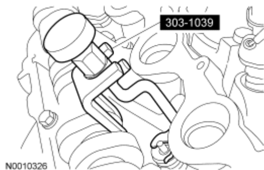
Fig. 336: Compressing Valve Spring With Special Tool Courtesy of FORD MOTOR CO.
