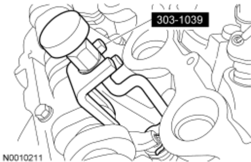
Fig. 127: Identifying Special Tool For Removing/Installing Camshaft Roller Followers Courtesy of FORD MOTOR CO.
