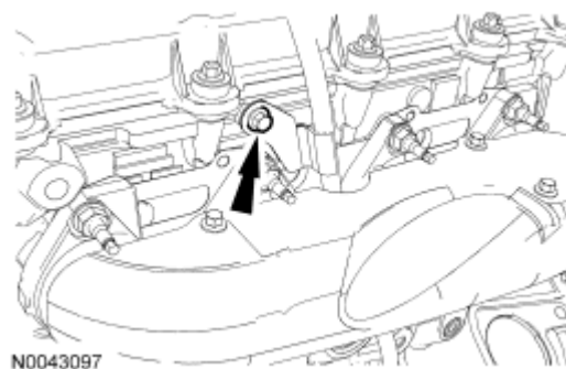
Fig. 222: Locating Oil Level Indicator Tube Bolt Courtesy of FORD MOTOR CO.
