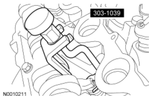
Fig. 140: Identifying Special Tool For Removing/Installing Camshaft Roller Followers Courtesy of FORD MOTOR CO.
