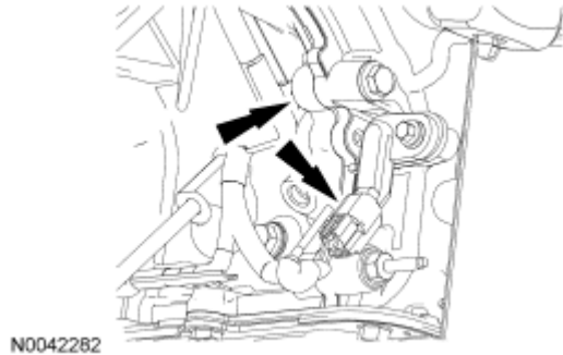
Fig. 433: Locating Crankshaft Position Sensor Electrical Connector And Wiring Harness Retainer Courtesy of FORD MOTOR CO.
