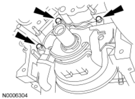
Fig. 329: Locating Oil Pump Bolts Courtesy of FORD MOTOR CO.
