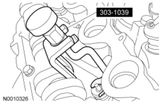
Fig. 138: Compressing Valve Spring With Special Tool Courtesy of FORD MOTOR CO.
