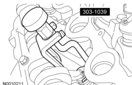
Fig. 235: Identifying Special Tool For Removing/Installing Camshaft Roller Followers Courtesy of FORD MOTOR CO.
