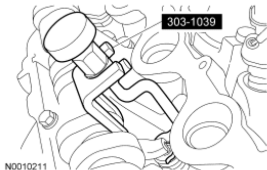
Fig. 145: Identifying Special Tool For Removing/Installing Camshaft Roller Followers Courtesy of FORD MOTOR CO.
