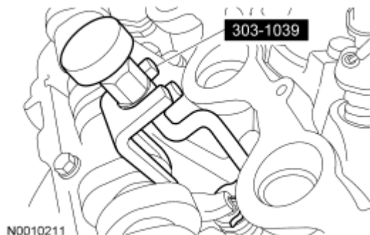
Fig. 310: Identifying Special Tool For Removing/Installing Camshaft Roller Followers Courtesy of FORD MOTOR CO.
