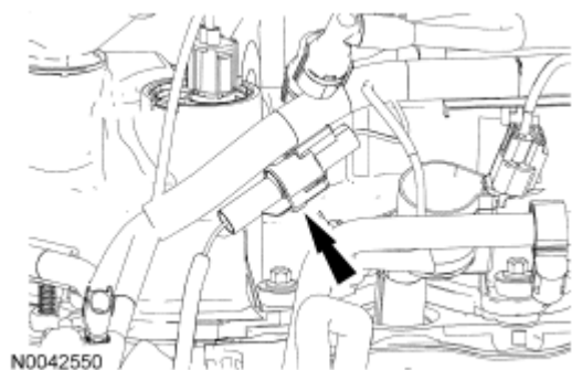
Fig. 474: Locating Electrical Connector Courtesy of FORD MOTOR CO.
