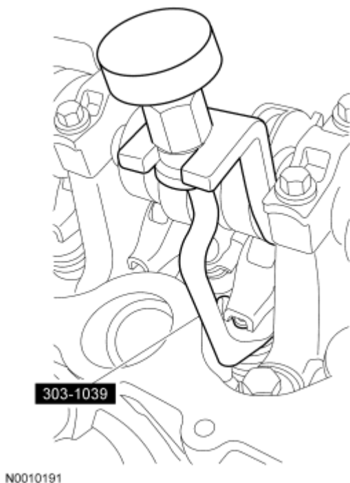
Fig. 104: Compressing Spring Using Special Tool Courtesy of FORD MOTOR CO.
