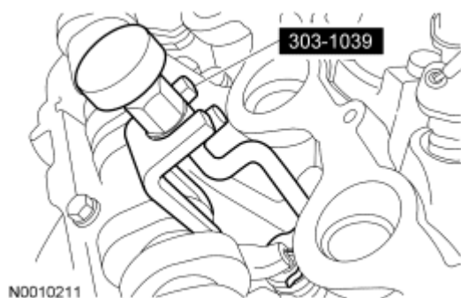
Fig. 137: Identifying Special Tool For Removing/Installing Camshaft Roller Followers Courtesy of FORD MOTOR CO.
