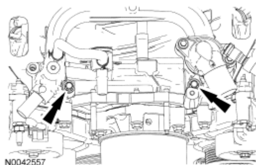
Fig. 182: Locating PCV Fitting Hose Assembly Bolts Courtesy of FORD MOTOR CO.
