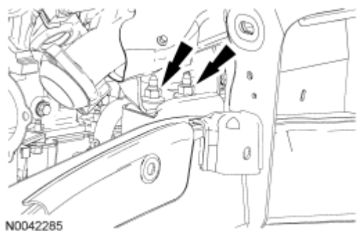
Fig. 449: Locating RH Engine Support Insulator Nuts Courtesy of FORD MOTOR CO.
