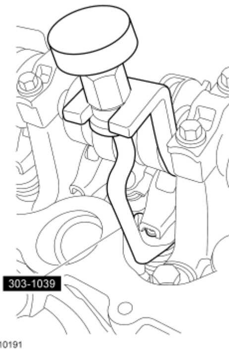
Fig. 237: Compressing Spring Using Special Tool Courtesy of FORD MOTOR CO.
