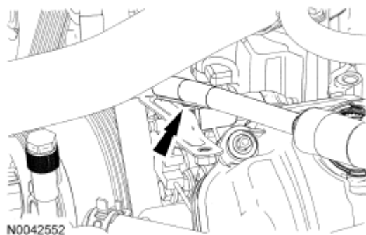
Fig. 189: Locating Wiring Harness Retainer From Cooling Fan Wiring Harness Bracket Courtesy of FORD MOTOR CO.
