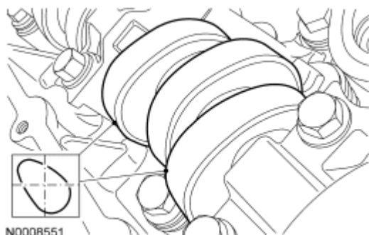
Fig. 246: Identifying Camshaft Lobe Position Courtesy of FORD MOTOR CO.
