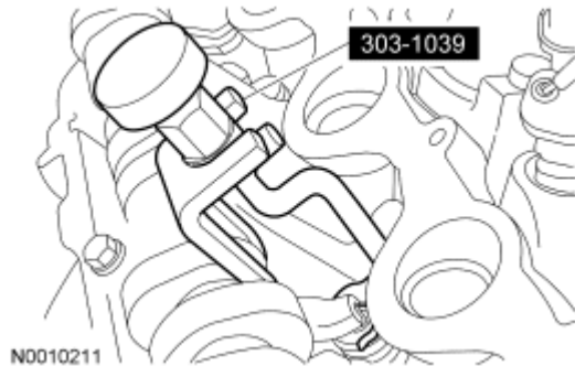
Fig. 134: Identifying Special Tool For Removing/Installing Camshaft Roller Followers Courtesy of FORD MOTOR CO.
