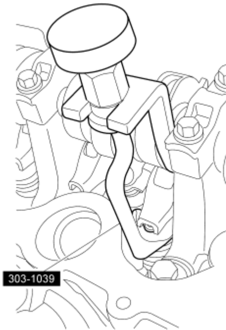
Fig. 397: Compressing Spring Using Special Tool Courtesy of FORD MOTOR CO.
