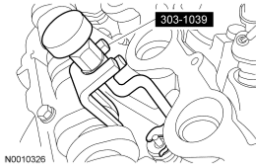
Fig. 133: Compressing Valve Spring With Special Tool Courtesy of FORD MOTOR CO.
