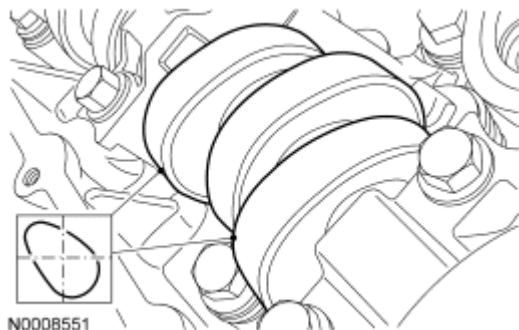
Fig. 120: Identifying Camshaft Lobe Position Courtesy of FORD MOTOR CO.
