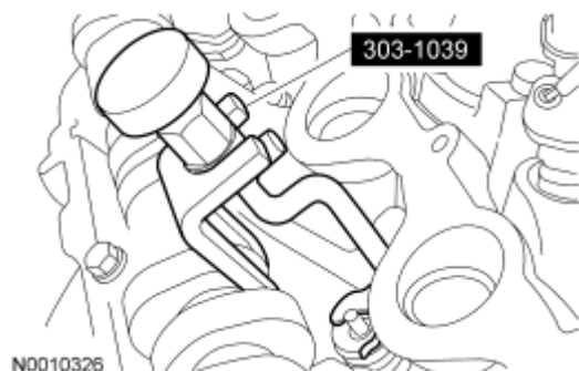
Fig. 350: Compressing Valve Spring With Special Tool Courtesy of FORD MOTOR CO.
