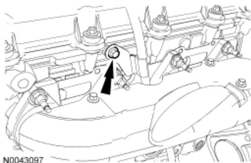
Fig. 536: Locating Oil Level Indicator Tube Bolt Courtesy of FORD MOTOR CO.
