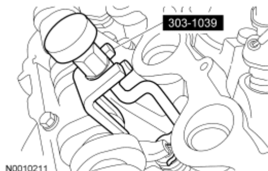
Fig. 324: Identifying Special Tool For Removing/Installing Camshaft Roller Followers Courtesy of FORD MOTOR CO.
