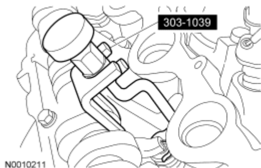
Fig. 135: Identifying Special Tool For Removing/Installing Camshaft Roller Followers Courtesy of FORD MOTOR CO.
