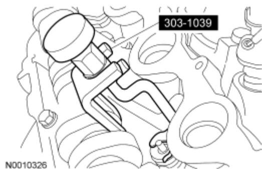
Fig. 132: Compressing Valve Spring With Special Tool Courtesy of FORD MOTOR CO.
