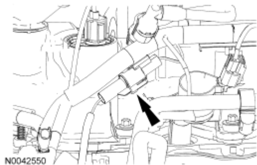
Fig. 187: Locating Electrical Connector Courtesy of FORD MOTOR CO.
