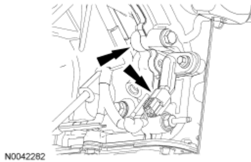
Fig. 279: Locating Crankshaft Position Sensor Electrical Connector And Wiring Harness Retainer Courtesy of FORD MOTOR CO.
