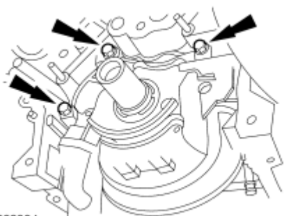
Fig. 368: Locating Oil Pump Bolts Courtesy of FORD MOTOR CO.
