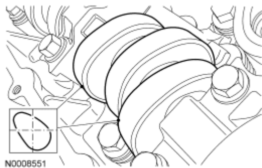
Fig. 44: Identifying Camshaft Lobe Position Courtesy of FORD MOTOR CO.
