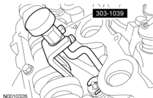
Fig. 352: Compressing Valve Spring With Special Tool Courtesy of FORD MOTOR CO.
