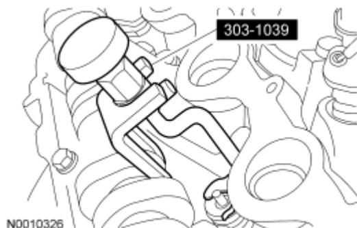
Fig. 354: Compressing Valve Spring With Special Tool
