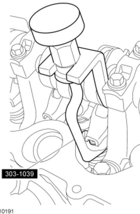
Fig. 401: Compressing Spring Using Special Tool Courtesy of FORD MOTOR CO.
