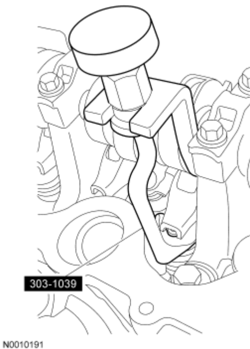
Fig. 99: Compressing Spring Using Special Tool Courtesy of FORD MOTOR CO.
