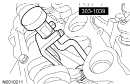
Fig. 326: Identifying Special Tool For Removing/Installing Camshaft Roller Followers Courtesy of FORD MOTOR CO.
