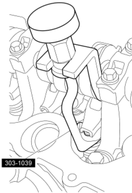
Fig. 86: Compressing Spring Using Special Tool Courtesy of FORD MOTOR CO.
