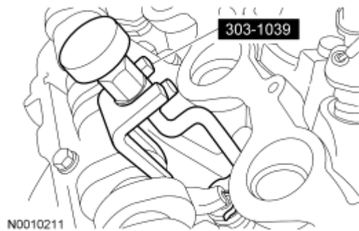
Fig. 108: Identifying Special Tool For Removing/Installing Camshaft Roller Followers Courtesy of FORD MOTOR CO.
