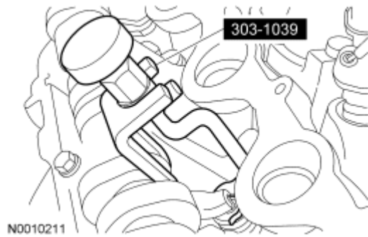
Fig. 130: Identifying Special Tool For Removing/Installing Camshaft Roller Followers Courtesy of FORD MOTOR CO.
