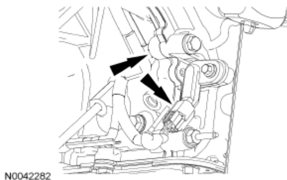
Fig. 281: Locating Crankshaft Position Sensor Electrical Connector And Wiring Harness Retainer Courtesy of FORD MOTOR CO.
