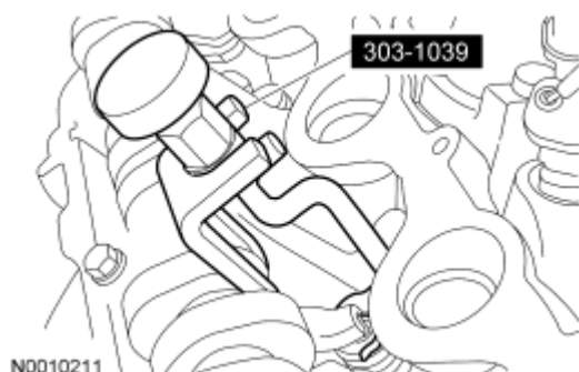
Fig. 121: Identifying Special Tool For Removing/Installing Camshaft Roller Followers Courtesy of FORD MOTOR CO.
