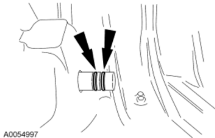
Fig. 504: Locating O-Ring Seals Courtesy of FORD MOTOR CO.
