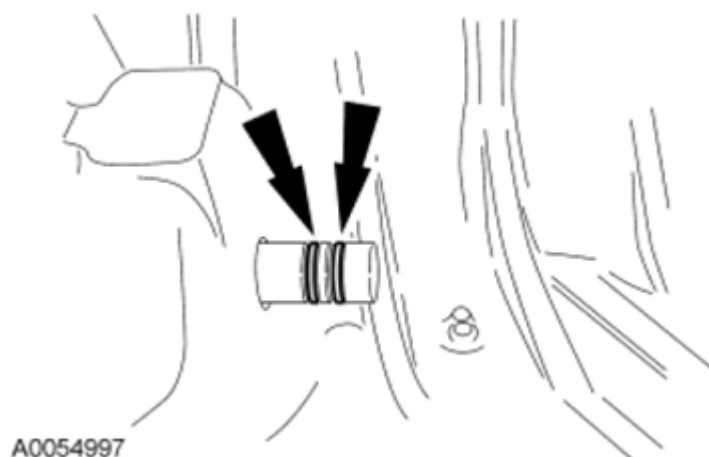
Fig. 413: Locating O-Ring Seals Courtesy of FORD MOTOR CO.
