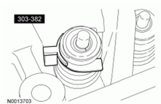
Fig. 332: Remove/Install Valve Spring Compressor Spacer Between Valve Spring Coils Courtesy of FORD MOTOR CO.
