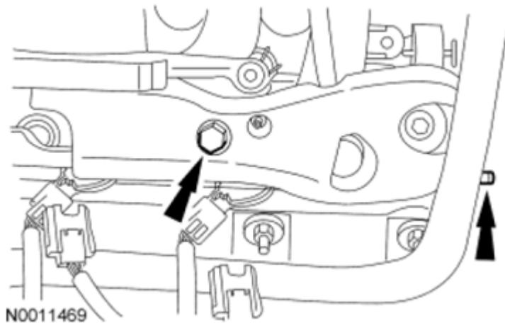
Fig. 419: Locating Crash Bracket And Mounting Bolt Courtesy of FORD MOTOR CO.
