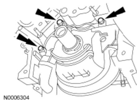
Fig. 355: Locating Oil Pump And Bolts Courtesy of FORD MOTOR CO.
