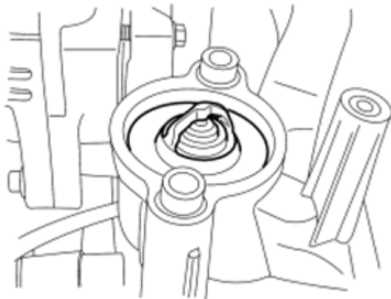
Fig. 511: Locating Thermostat And O-Ring Courtesy of FORD MOTOR CO.
