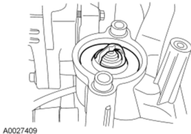
Fig. 420: Locating Thermostat And O-Ring Courtesy of FORD MOTOR CO.
