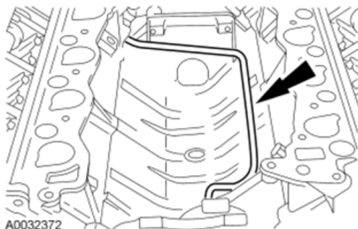
Fig. 505: Locating Coolant Bypass Tube Courtesy of FORD MOTOR CO.
