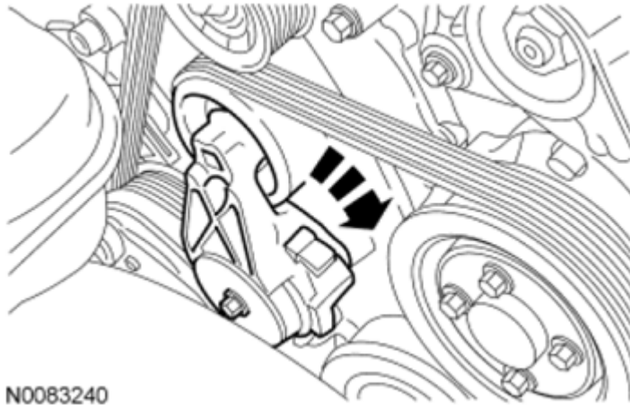
Fig. 93: Rotating Tensioner Clockwise Courtesy of FORD MOTOR CO.
