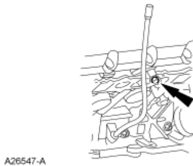
Fig. 195: Locating Oil Level Indicator Tube Mounting Bolt Courtesy of FORD MOTOR CO.
