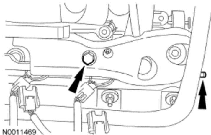
Fig. 510: Locating Crash Bracket And Mounting Bolt Courtesy of FORD MOTOR CO.
