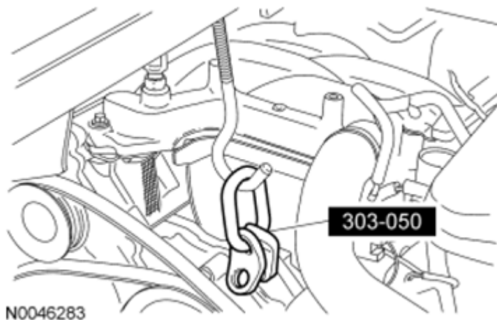
Fig. 142: Installing Engine Lifting Bracket Courtesy of FORD MOTOR CO.
