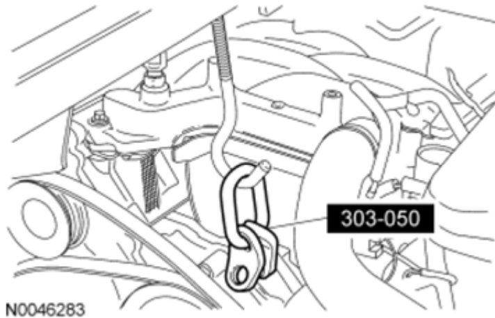
Fig. 138: Installing Engine Lifting Bracket Courtesy of FORD MOTOR CO.
