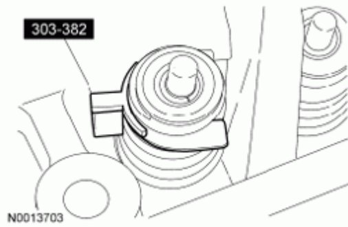
Fig. 87: Remove/Install Valve Spring Compressor Spacer Between Valve Spring Coils Courtesy of FORD MOTOR CO.
