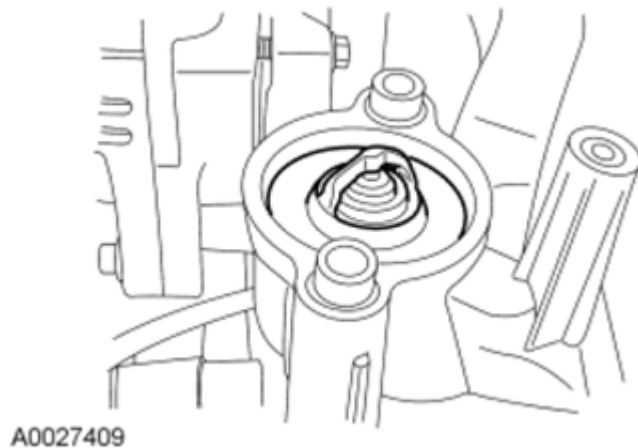
Fig. 273: Locating Thermostat And O-Ring Courtesy of FORD MOTOR CO.
