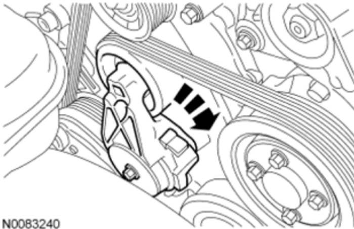
Fig. 25: Rotating Tensioner Clockwise Courtesy of FORD MOTOR CO.
