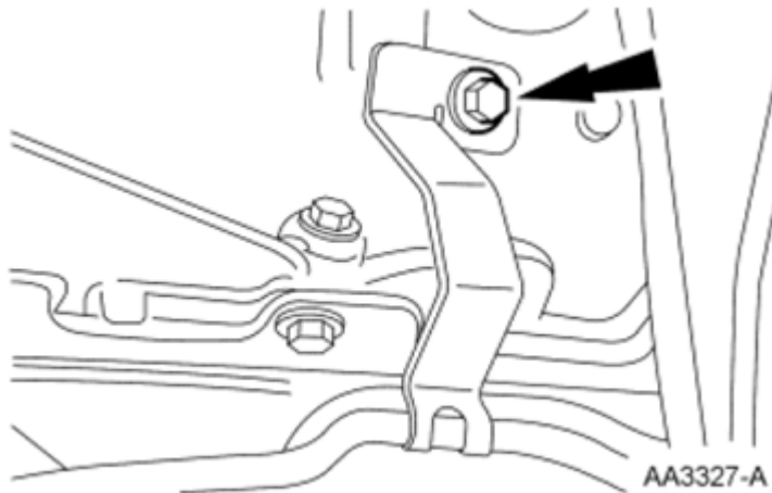
Fig. 555: Locating Transmission Oil Cooler Tube Bracket Bolt Courtesy of FORD MOTOR CO.
