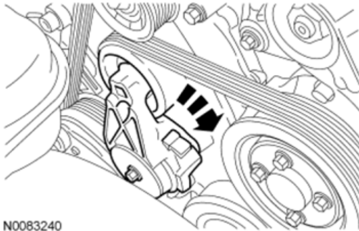
Fig. 93: Rotating Drive Belt Tensioner Clockwise Courtesy of FORD MOTOR CO.
