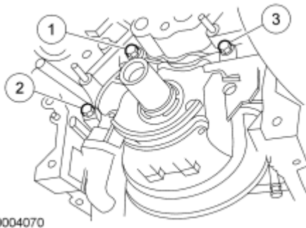
Fig. 347: Identifying Oil Pump Bolts Tightening Sequence Courtesy of FORD MOTOR CO.
