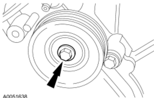
Fig. 281: Accessory Drive Belt Idler Pulley Bolt Courtesy of FORD MOTOR CO.
