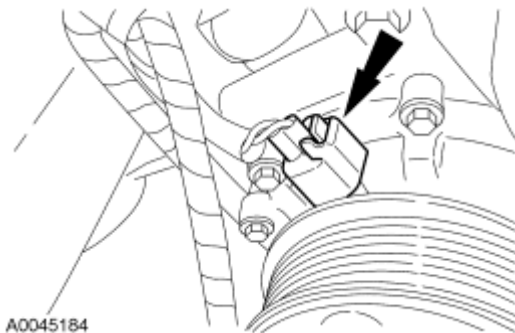
Fig. 551: A/C Compressor Electrical Connector Courtesy of FORD MOTOR CO.
