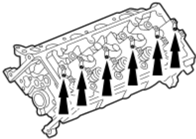
Fig. 322: Camshaft Journals Courtesy of FORD MOTOR CO.
