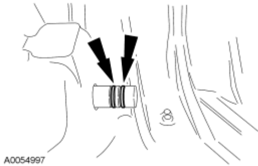
Fig. 502: O-Ring Seals Courtesy of FORD MOTOR CO.
