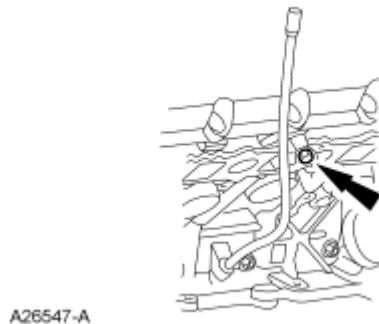
Fig. 195: Locating Oil Level Indicator Tube Bolts Courtesy of FORD MOTOR CO.
