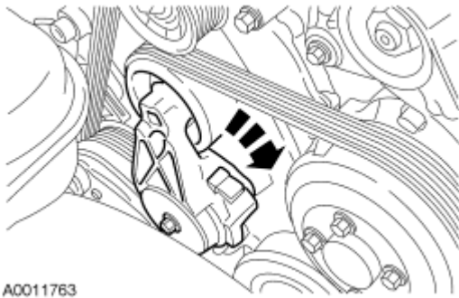
Fig. 94: Rotating Tensioner Clockwise Courtesy of FORD MOTOR CO.
