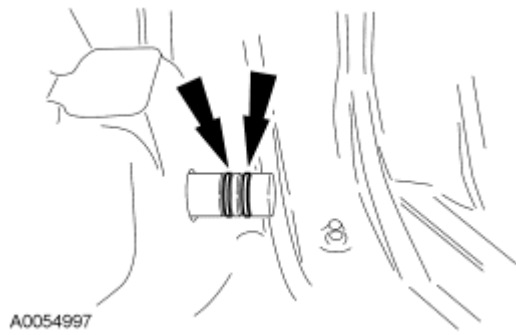
Fig. 410: O-Ring Seals Courtesy of FORD MOTOR CO.
