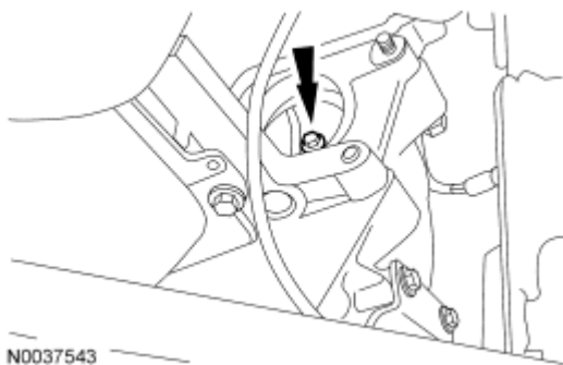
Fig. 543: Torque Converter Nut Courtesy of FORD MOTOR CO.
