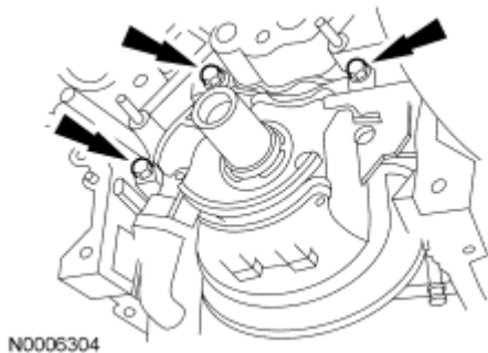
Fig. 307: Locating Oil Pump Bolts Courtesy of FORD MOTOR CO.
