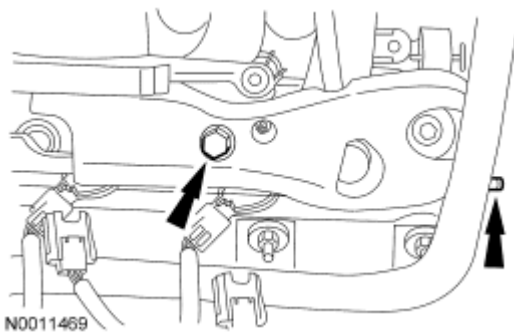
Fig. 415: Intake Manifold Crash Bracket Bolt Courtesy of FORD MOTOR CO.
