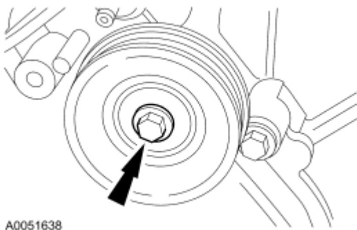
Fig. 404: Accessory Drive Belt Idler Pulley Bolt Courtesy of FORD MOTOR CO.
