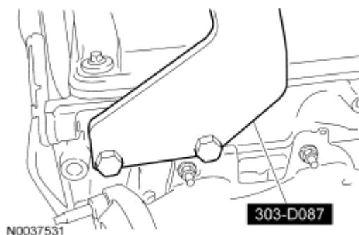
Fig. 122: Installing Special Tool To RH Cylinder Head Courtesy of FORD MOTOR CO.
