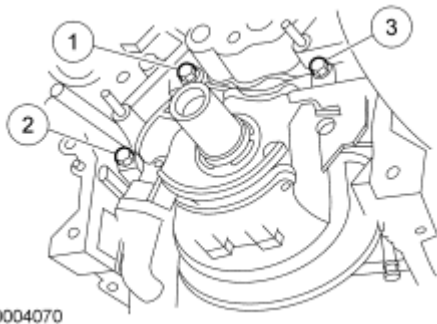
Fig. 353: Identifying Tightening Sequence Of Oil Pump Bolts Courtesy of FORD MOTOR CO.
