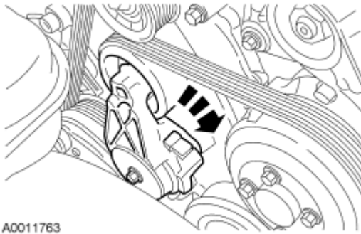
Fig. 24: Rotating Tensioner Clockwise Courtesy of FORD MOTOR CO.
