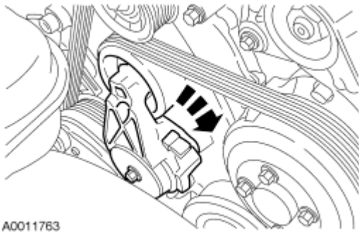
Fig. 92: Rotating Tensioner Clockwise Courtesy of FORD MOTOR CO.
