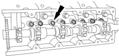
Fig. 303: Locating Hydraulic Lash Adjusters Courtesy of FORD MOTOR CO.
