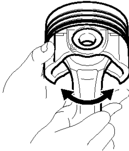
Fig. 205: Checking Fitting Condition Between Piston And Piston Pin Courtesy of TOYOTA MOTOR SALES, U.S.A., INC.
