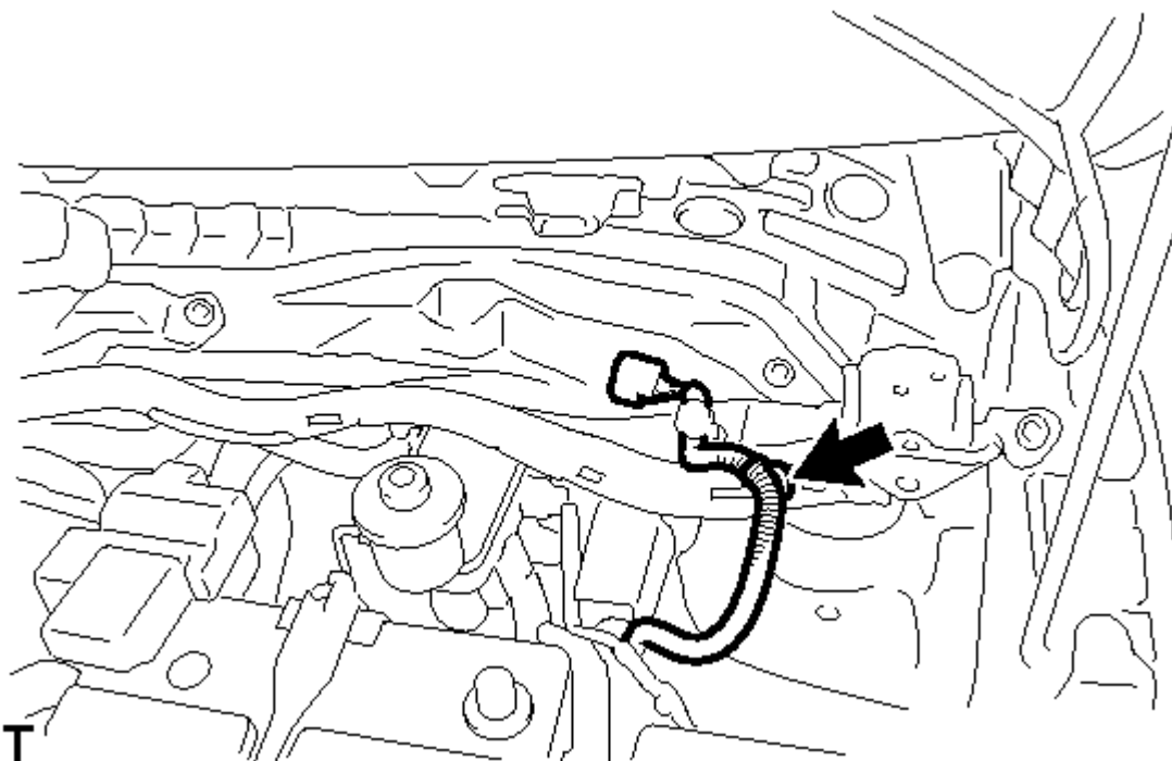
Fig. 335: Identifying Wire Harness Clamp Courtesy of TOYOTA MOTOR SALES, U.S.A., INC.
