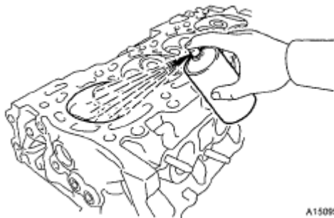
Fig. 114: Inspecting Cylinder Head For Cracks Courtesy of TOYOTA MOTOR SALES, U.S.A., INC.
