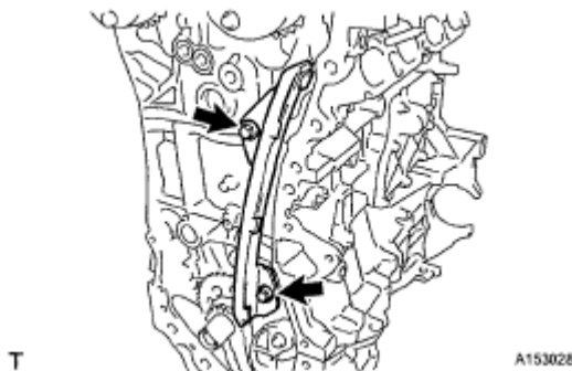
Fig. 511: Locating No. 1 Chain Vibration Damper And Bolts Courtesy of TOYOTA MOTOR SALES, U.S.A., INC.
