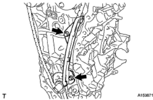
Fig. 401: Locating Bolts And Chain Vibration Damper Courtesy of TOYOTA MOTOR SALES, U.S.A., INC.
