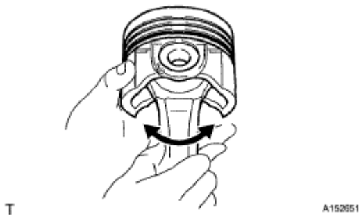
Fig. 205: Checking Fitting Condition Between Piston And Piston Pin Courtesy of TOYOTA MOTOR SALES, U.S.A., INC.
