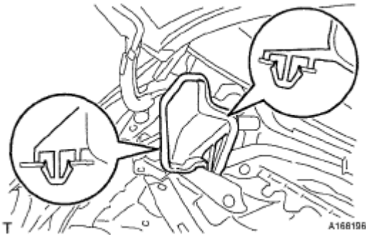
Fig. 336: Identifying Claws Locations Courtesy of TOYOTA MOTOR SALES, U.S.A., INC.
