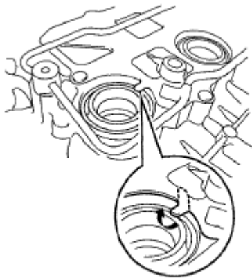
Fig. 464: Identifying Claws Of Baffle Plate Courtesy of TOYOTA MOTOR SALES, U.S.A., INC.
