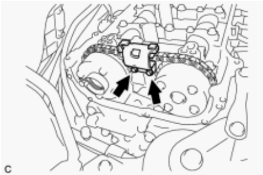
Fig. 56: Identifying Chain Vibration Damper
