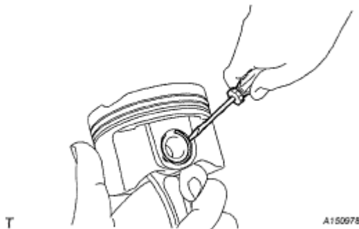
Fig. 163: Prying Out Snap Rings
