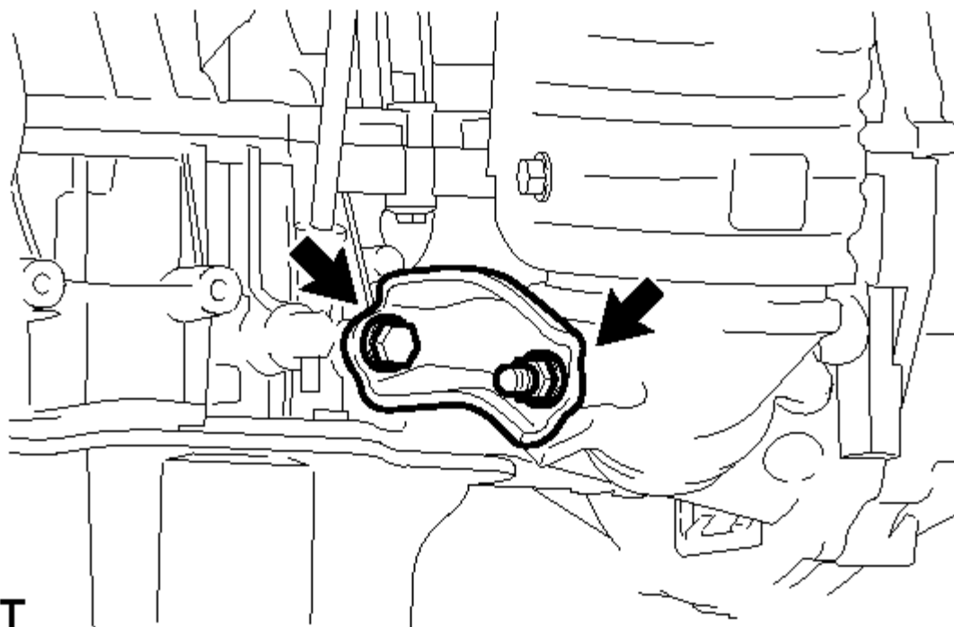
Fig. 362: Locating Manifold Stay Components Courtesy of TOYOTA MOTOR SALES, U.S.A., INC.
