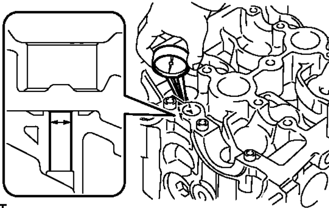
Fig. 176: Measuring Bush Bore Diameter Of Cylinder Head
